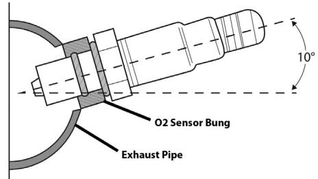
2. Mark the drilling location on the exhaust system pipe with a permanent or paint marker. Check the proposed mounting location to ensure the clearance for the O2 sensor is adequate and that the O2 sensor connector on the main harness will reach the O2 sensor location. Make sure to take engine movement into consideration when checking for clearance.
