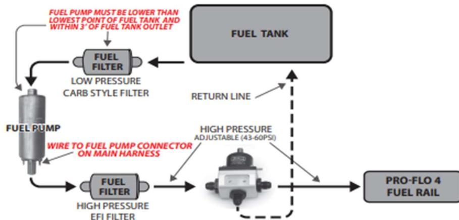
**Part Number 36031 Universal EFI Fuel Sump System:** Equipped with an internal 67 GPH (255 LPH) fuel pump and adjustable fuel pressure regulator. Uses engines stock mechanical fuel pump to provide fuel to the internal high pressure EFI fuel pump.
