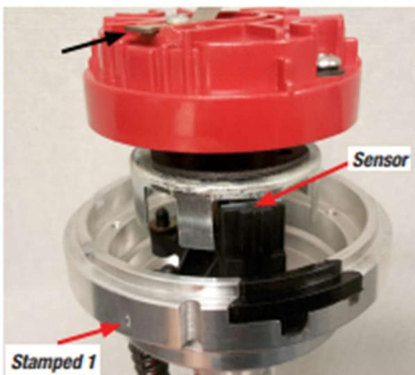
5. Install the spark plug wires. Position cylinder 1 spark plug wire on the distributor cap post located at the 1 stamped on the distributor housing.
