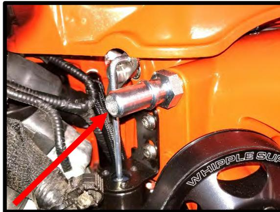
109. Install the supplied PCV hose to the passenger side valve cover. Connect other end to the supercharger inlet quick connect fitting. Push until it clicks and locks into place.
