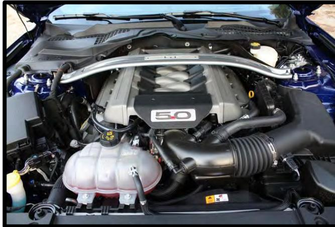
18. Remove the factory plastic engine cover from the engine by pulling up.
