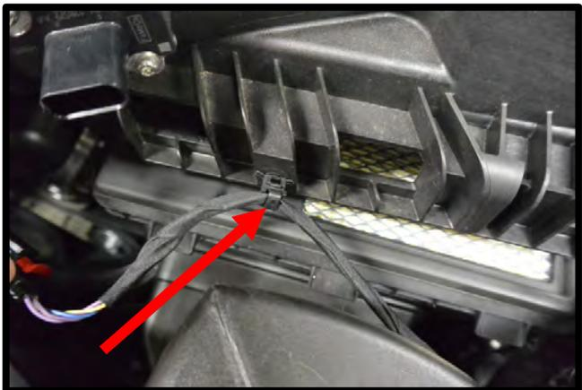
22. Detach the sound box from airbox. Remove the bolts securing airbox to vehicle, lift and remove airbox from vehicle.
