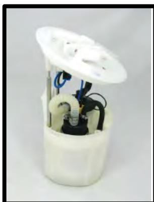
164. **(Stage 2)** Reinstall the assembly into the fuel tank and attach a length of hose to the outlet of the pump assembly allowing it to drain into a fuel safe container and prime the fuel pump assembly. Attach the supply line to the outlet of the pump assembly.
