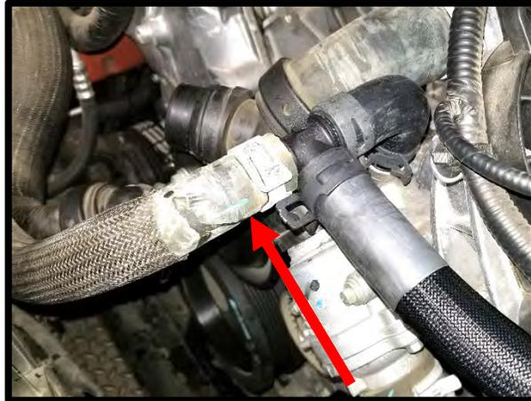
59. Remove upper radiator hose from radiator. Use a hose cutter, remove 1" from the radiator hose end. Reinstall hose once completed and secure with factory hose clamp. **TIP:** This is for added clearance for the new belt system.
