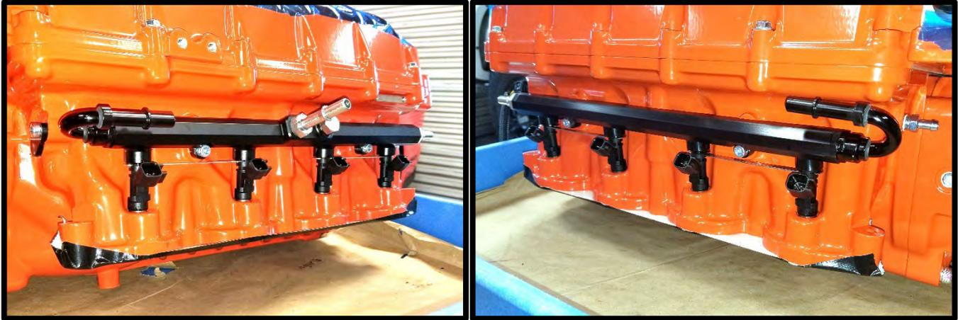
82. Install the supplied 3/8" fuel cross over line around the back of the supercharger by pressing until they click and lock in place. It's also possible to leave off until after SC is installed for easier access to rear bolts. **\*Note:** The 90deg end goes to bank 2 side.
