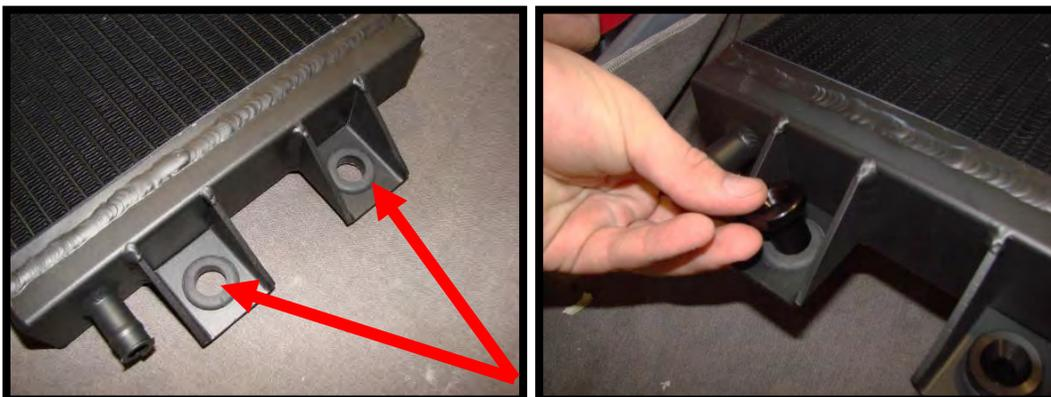
119. Install the LTR brackets to the LTR using the supplied (4) 8mm x 35mm FHSCS bolts through the aluminum heat exchanger spuds (5mm allen socket). **NOTE:** HD heat exchanger mounts the same way but the inlet fitting moves to RH side (same as outlet).
