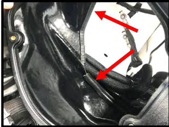
143. Install the supplied lower airbox to the vehicle by slipping over the factory air duct. Make sure the 3/4" and 3/8" IC tank to filler tee hoses go in the allotted area. These should be zip-tied together for clean installation and free of any kinks.
