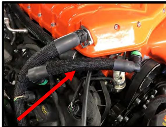
110. **(Complete kits)** Connect the previously routed Manifold Charge Temperature pigtail to the MCT sensor located in the back of the intake manifold.
