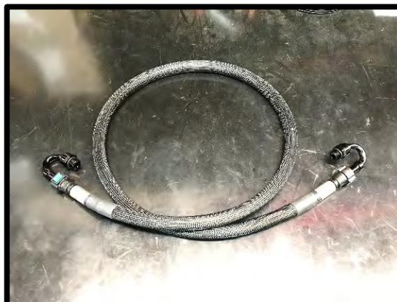
84. Install the supplied ¼" ID bypass actuator to the bypass nipple and ¼" nipple on SC housing. **CAUTION:** Do not open/close bypass actuator by hand. This may damage actuator internally. It only moves properly with equal vacuum/boost at the actuator reference port. **NOTE: Install zip tie to 90deg rubber fitting on bypass actuator nipple to secure, failing to do so may end with the hose coming off during WOT operation.**
