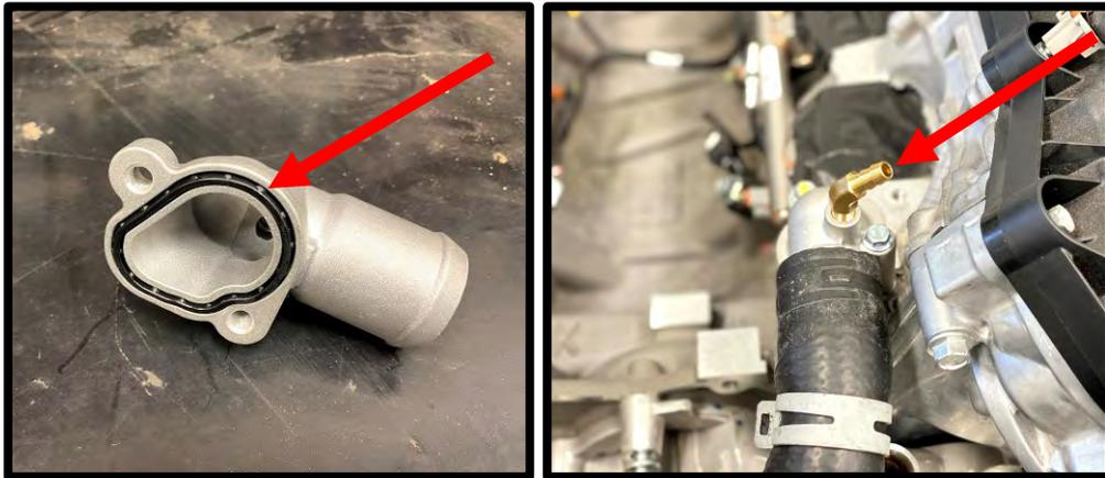
56. Using needle nose pliers, rotate the factory pinch clamp at the water neck towards the driver side for future clearance of the SC. **NOTE:** Image shows clamp with SC installed to illustrate max clearance.
