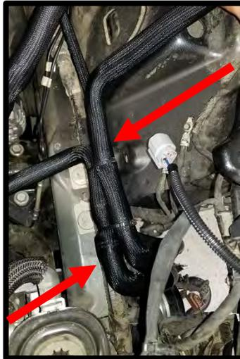
137. Install the supplied 3/4" ID molded hose (enclosed air kit hose #18MST-1001A) (open air kit hose #18MST-1001) from the IC **OUT** fitting to the airbox area for later installation. Secure end with supplied worm clamp. **TIP: The (2) hoses on this side should match in shape/form, therefore ensure it fits correctly. CAUTION: For hood clearance, ensure that the nut of the clamp is not on top.**
