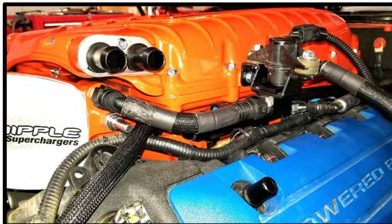
106. Install the supplied 3/8" x 20 1/2" hose with dual 90deg 9.49mm quick connect fittings from the EVAP solenoid rear fitting to the EVAP fitting located under the brake booster.
