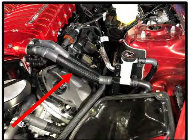
151. Install the supplied 3/8" ID x 31 1/2" IC vent line (COYO-1400) and the 3/4" ID x 24 1/2" IC rubber hose (COYO-1300) to the filler neck. Both use the 90deg on the filler tee. Secure both with supplied pinch clamps. Route both below the airbox, to the IC reservoir. Secure both ends with supplied pinch clamps. Use multiple zip-ties to secure hoses together. **Watch for hose kinks!**
