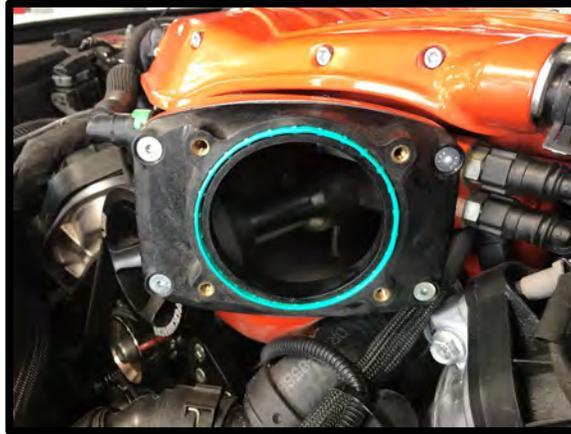
140. **(Stage 1)** Remove stock TB from intake manifold using 10mm socket. Install the stock throttle body using the (4) 6mm x 50mm FHSCS bolts using a 10mm socket. Connect throttle extension harness until it locks in place.
