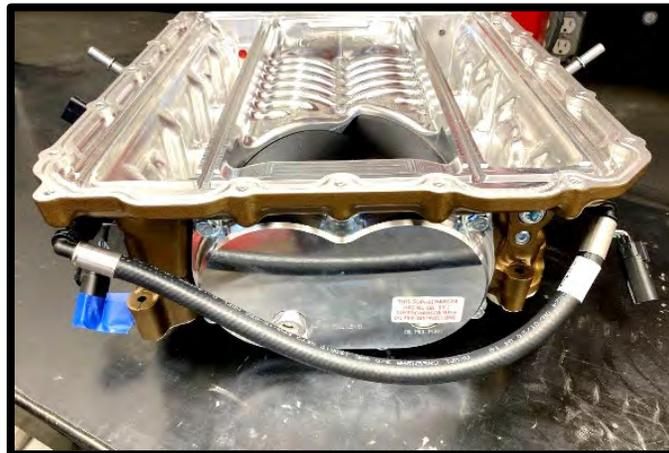
83. Route the supplied 3/8" x 50" cross over fuel hose around the back of the supercharger. (2) Adel clamps are supplied to secure to 2 SC Lid bolts across the back when installing lid later.
