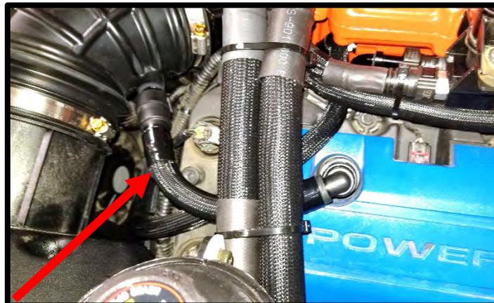
155. Connect the previously routed 1/4" vent line to the stock overflow tank, secure with stock clamp. Secure this hose to the radiator hose and heater hose using multiple zip-ties.
