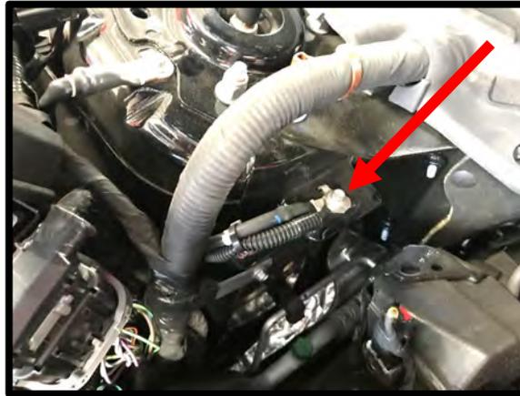
62. Open fuse box lid. Using a 10mm socket, remove the 12V (+) power stud nut from the far post. Install the IC pump relay power eyelet (red wire) to the 12V stud. Use a 10mm socket to secure stock and IC power wire.
