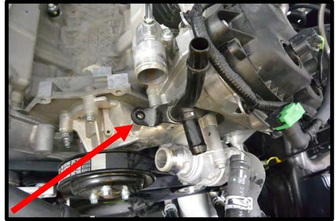
48. Loosen the (3) bolts securing the water pump pulley (while belt is on) using a 10mm socket. Remove the belt from the engine by using a 15mm socket on a 1/2" breaker bar and rotating the spring-loaded tensioner in a clockwise direction. Remove the spring-loaded tensioner from the engine using a 13mm socket (bolt will be reused later). Using 10mm socket, remove water pump pulley from engine (will be reused later).
