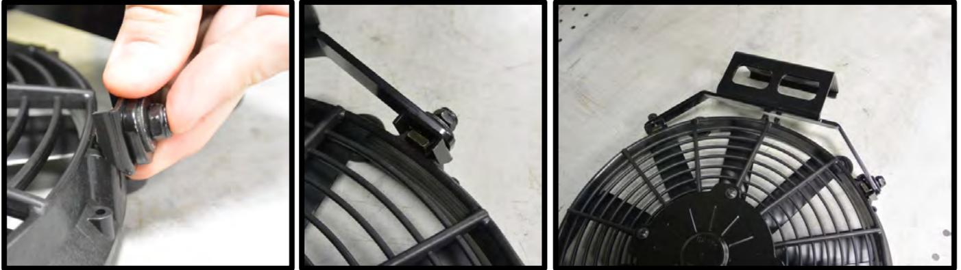
115. **(Dual fan installation)** Carefully set both fan assemblies on top front of the LTR, space these evenly before installing.
