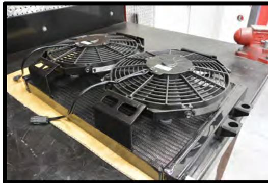
116. **(Dual fan installation)** Carefully pull open brackets and push onto the LTR. Its best to do both ends at the same time otherwise the bracket can be at an angle and hard to get on. **NOTE:** Electrical connectors should face down.
