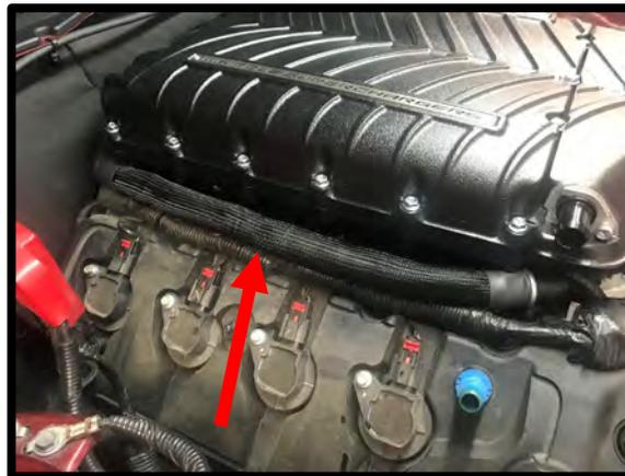
52. Install the supplied plastic heater tubes. Install the supplied oring to the tube and apply light amount of grease to oring surface. Install tube into block, then secure locking bracket with the factory bolt using an 8mm socket. **NOTE:** The bracket and heater tube has one locking tang, ensure they are lined up during installation. Torque to 89 lbs-in.
