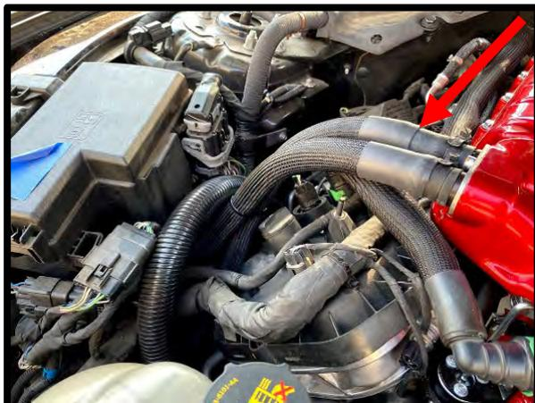
134. Install the supplied preformed  $\frac{3}{4}$ " x 48" hose to upper Y-fitting and secure with constant tension clamp. The straight end goes to the Y. Route between the engine and radiator to LH side of vehicle. Leave this end loose until airbox installation. Secure hose to factory heater lines using zip-ties. **NOTE:** Failure to secure line will result in hose hitting belt system.
