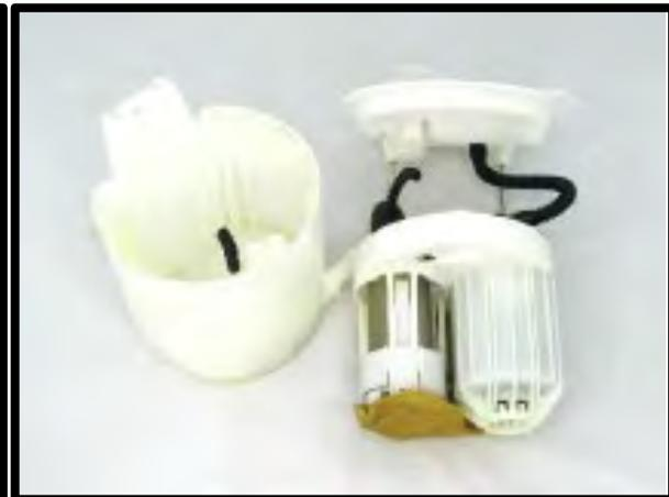
158. **(Stage 2)** Carefully cut the larger pump outlet hose (3/8" ID) from the assembly filter and remove the OE pump.
