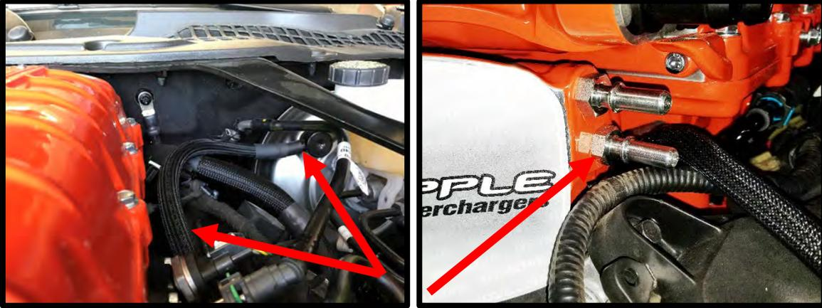
108. Install the (1) supplied -6AN viton oring (#906) to the (1) -6 ORB to 15.82mm quick connect fittings. Install this fitting to the RH side 6AN fittings on the inlet using a 7/8" wrench.
