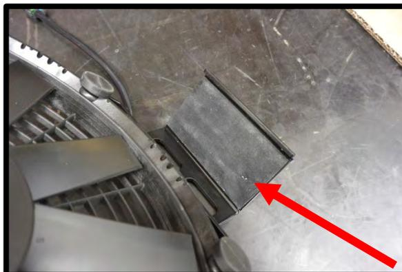
114. **(Dual fan installation)** Install the (4) brackets to the fans by sliding the square tab into the fan notch and the steel channel bracket will slide on the outside. The angled side will face the fan. This slides together easier if the bracket is facing slightly up. Once these are lined up, push until the seat together. Repeat on the other (3) brackets. Leave nyloc nuts loose for now.
