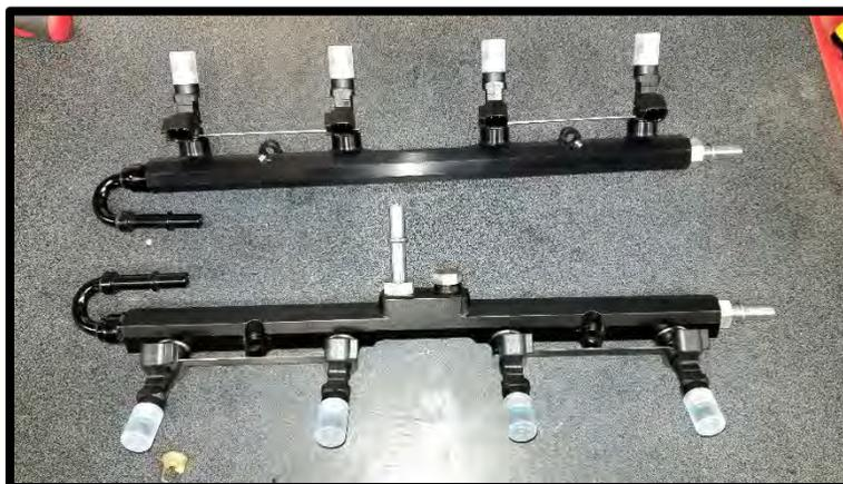
81. Apply generous amount of grease to the injector orings for ease of installation. Install the fuel injectors, rails and lock bracket to the intake manifold, secure with the (4) 6mm x 16mm SHCS using a 5mm allen socket. Torque to 90 lbs-in.
