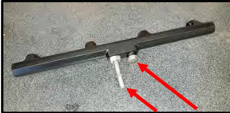
79. Install supplied (2) #2-906 orings to the (2) 9.49mm to -6 ORB inlet/outlet fittings. Install these (2) fittings into rear side of fuel rails. Apply light amount of grease to oring for ease of installation. Using a  $\frac{3}{4}$ " wrench (or  $\frac{3}{4}$ " deep socket) on both the front and rear fittings, tighten both. Install the (2) supplied 6AN 180deg swivel fittings to front port on each rail. Using a  $\frac{3}{4}$ " wrench, secure fittings to fuel rails.
