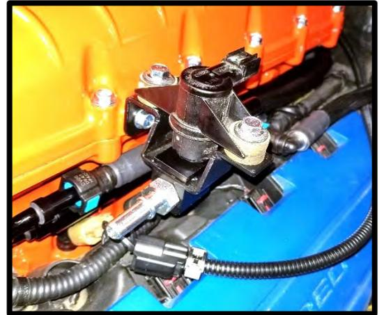
105. Install the supplied 3/8" ID x 4 1/2" hose to the EECPV barb fitting and **upper** quick connect fitting (55 Deg) on SC inlet. Push until it clicks and locks into place.
