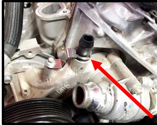
53. Install the supplied tee and 90deg hose to the driver side heater tube you just installed. Secure with supplied constant tension clamp on the 90deg hose to heater tube.
