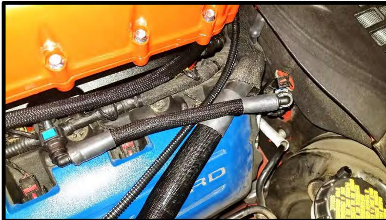
103. Install the (2) supplied 6AN viton oring (#906) to the (2) -6 ORB to 9.89mm quick connect fittings. Install these fittings to the passenger side lower 6AN fittings on the inlet using an 11/16" socket.
