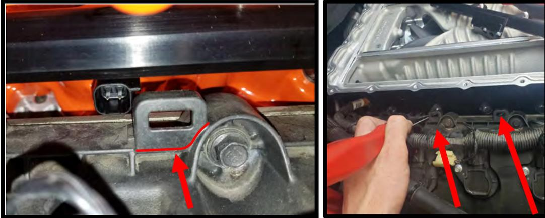
89. Install the supercharger housing (without lid) to the engine. Use the supplied (4) 6mm x 55mm HHFCS on the outer bolt holes and (6) 6mm x 80mm HHFCS bolts with the supplied (6) #2-009 orings on the bolt, under the head. Use **Blue Loctite #243** on the threads of each bolt. Leave hand tight for now.
