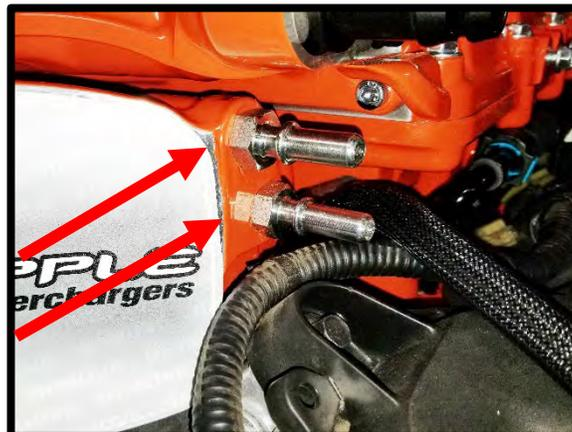
104. Install the EVAP to the supplied billet adapter with the electrical connector facing the back of engine. Install the supplied 9.89mm quick connect fitting and 6AN oring to billet adapter. Secure supplied EVAP bracket to the supercharger lid using the supplied (2) 6mm x 10mm HHFCS bolts. Secure EVAP assembly to bracket using the supplied (2) 6mm x 20mm HHFCS bolts.
