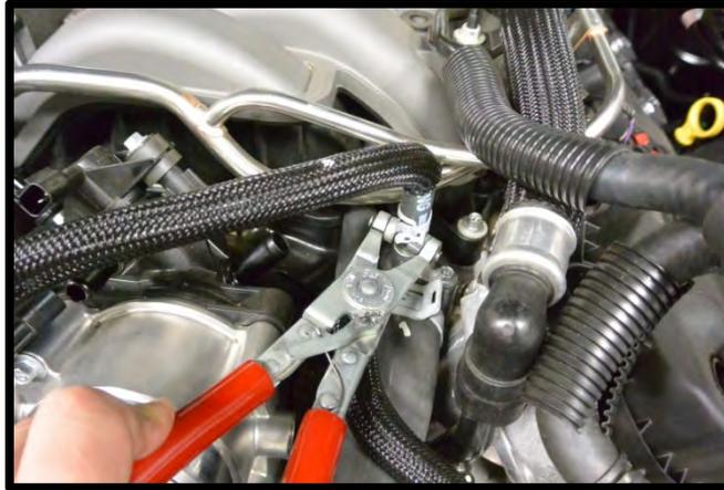
33. Remove the heater hoses from coolant tubes and push aside.
