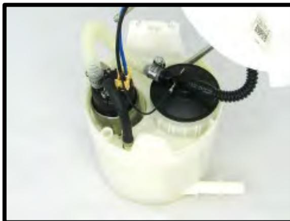
163. **(Stage 2)** Reinstall the hat to the assembly in the center/buckets assemblies and connect the electrical connector harness to the hat assembly.
