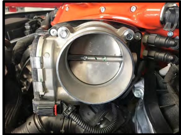
141. **(Stage 2 Whipple 132mm Crusher throttle body)** Install throttle body to supercharger inlet, use the supplied gasket between TB adapter and SC inlet. Secure with the supplied (3) 6mm x 25mm SHCS and (1) 6mm x 50mm SHCS using a 5mm allen socket. Torque to:
