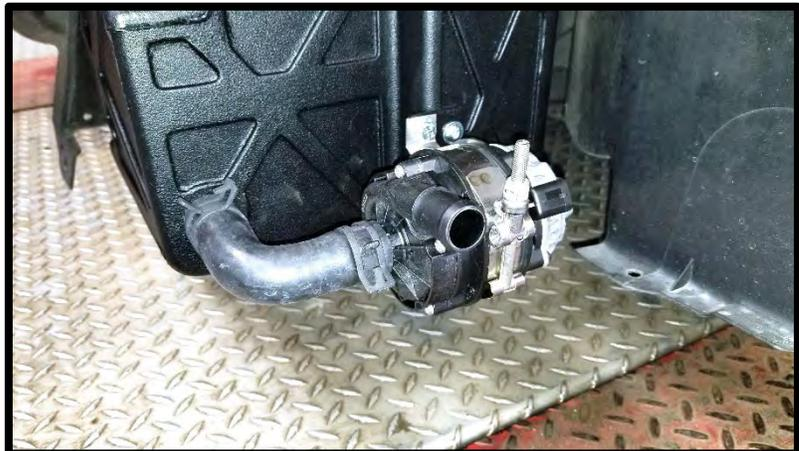
128. Install the supplied 180deg hose to the IC pump outlet. Route to LTR LH inlet fitting. Secure with constant tension clamps.
