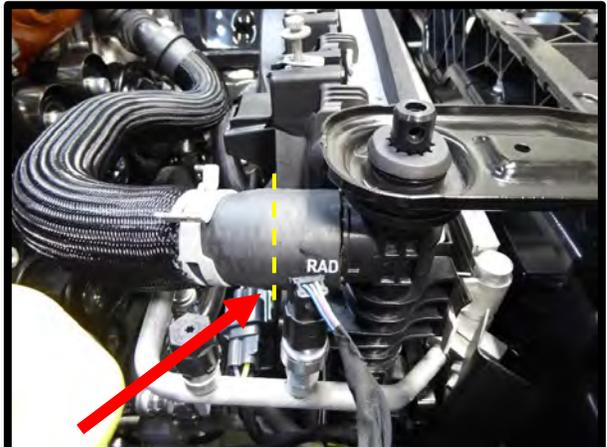
60. Remove coolant vent hose from the radiator and pull back the plastic sheaving. Shorten this hose end by 1" for additional clearance. Reinstall hose using factory clamp.
