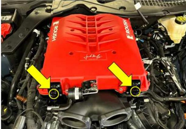
105. Verify top and bottom ports of the supercharger shown below. Note: To verify ALL hose connections, go to the last page of the manual and see the supercharger assembly - hose diagram.
