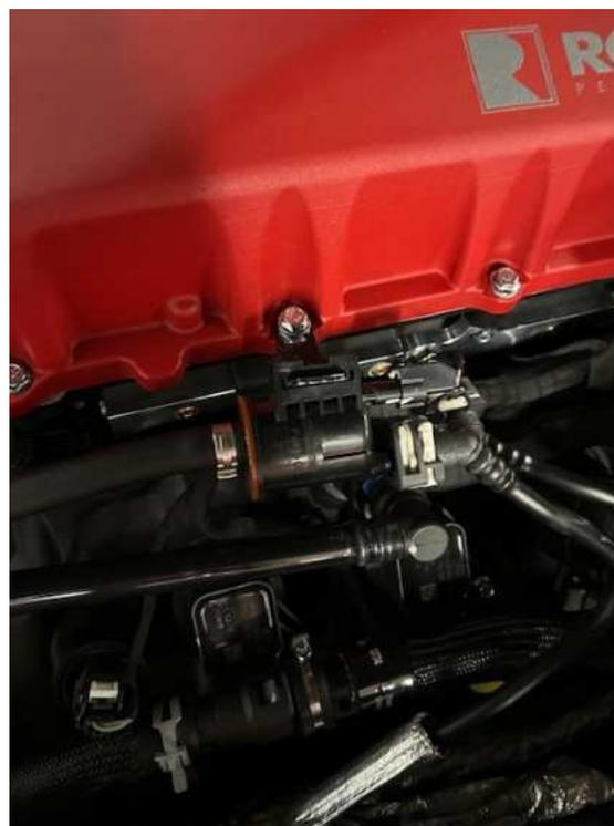
139. Route the EVAP hose to the barb on the left-hand side (driver side) of the supercharger inlet using EVAP hose clamp (Item 35, page 10) from hardware kit 31-26-50-029.
