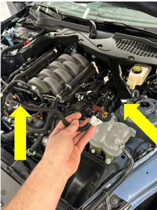
20. Disconnect the fuel rail supply and outlet line to the DI pump. Make sure to cover the fitting with rags and wear safety glasses and gloves to perform this step. **This step should only be attempted on a cold engine that has had the fuel pressure released already.**
