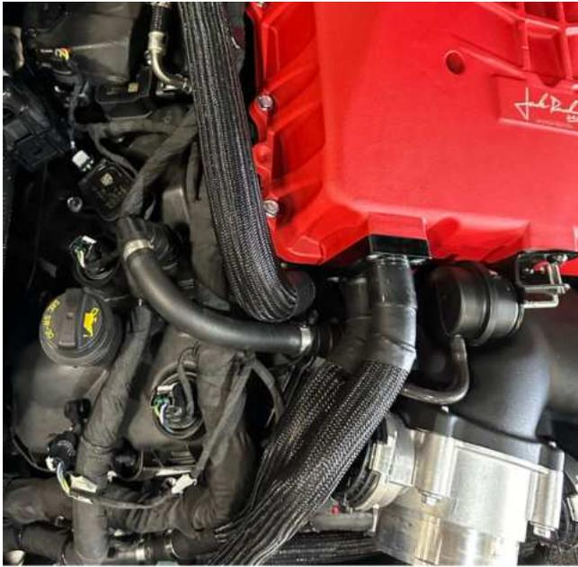
99. Install the bypass hose onto the 90 degree fitting on the right-hand side (passenger side) of the supercharger.
