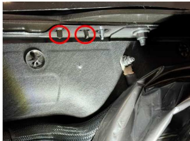
46. For Auto cars only: Locate the transmission fluid heater coolant control valve bracket from page 21 step 41. Modify the bracket as shown. Remove the valve from the bracket and cut the mount shown. Note: The lower leg will be removed from the valve mount. Spray black paint on cut area to prevent corrosion. Save part for re-use.
