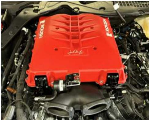
89. Connect the electrical connectors from both sides of the engine harness that goes to the throttle bodies. Note: left hand side (driver side) requires tape removal from the harness to spin the connector around.
