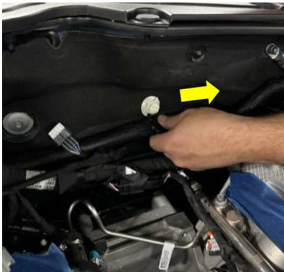
31. Obtain the provided 2 P-clips (Item 37, page 10) from hardware kit 31-26-50-029. Use them to mount the left-hand side (driver side) heater hose onto the coils as shown.
