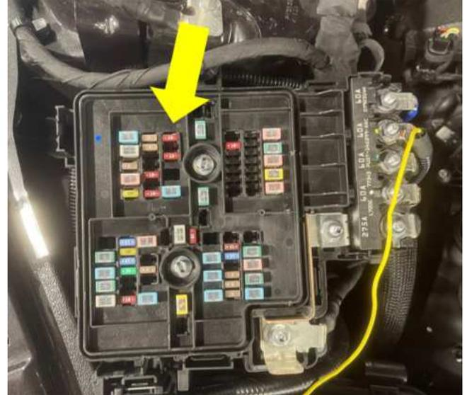
120. Route the intercooler electrical harness ground terminal to the ground bolt on the passenger fender under the air box as shown. Install the ground to the location shown. (8mm socket)
