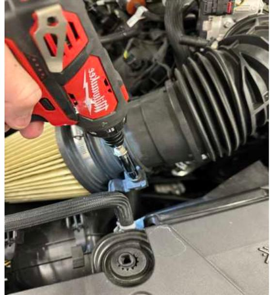
16. Disconnect both throttle body electrical connectors. Remove the 8 throttle body bolts (8mm socket) and remove both throttle bodies. Remove the throttle body harness retainers from the intake manifold. Save all parts for re-use.
