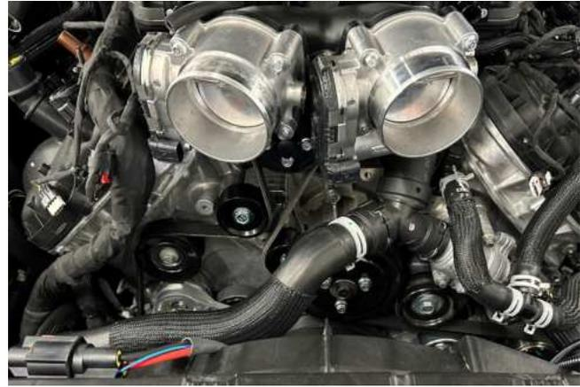
87. Install the supercharger lid onto the supercharger manifold. Use the 18 bolts removed in step 75. Torque bolts to 12 Nm. Note: Torque sequence is shown below.
