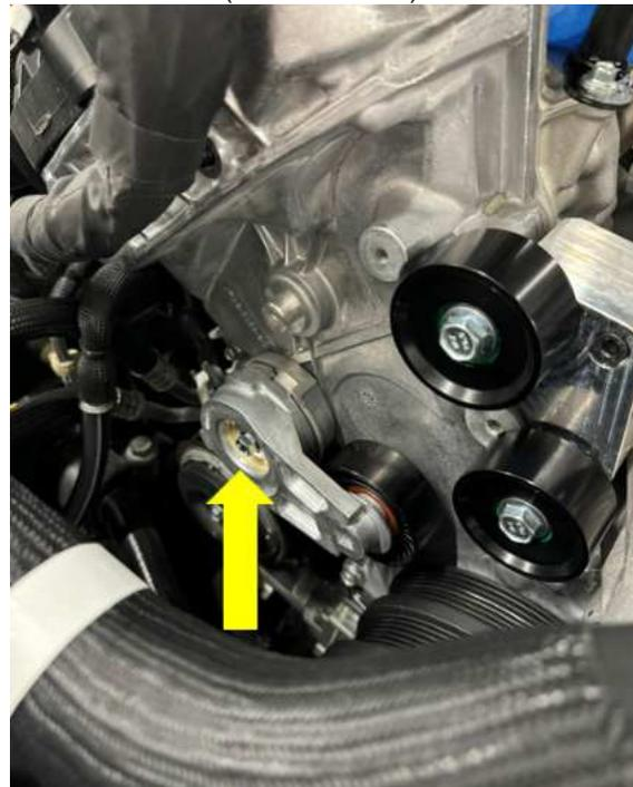
5. Install the ribbed idler pulley assembly (pulley and bolt) (Item 20, page 5) from hardware kit 31-26-50-025 into the location shown. Torque the bolt to 25Nm. (10mm socket)
