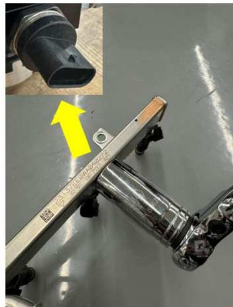
37. Gather the supplied copper washer (Item 50, page 10) from the hardware kit 31-26-50-029, it will be installed onto the pressure sensor as shown. Install it onto the open fuel rail port on the left-hand side (driver side) of the ROUSH intake manifold. (Lower part of the supercharger assembly) Torque to 40 Nm. (1-1/8" deep well socket)
