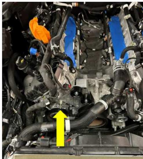
41. For Auto cars only: Remove the transmission fluid heater coolant control valve bracket. This is located on the right-hand side front cover. Keep bracket and hardware for reinstall.
