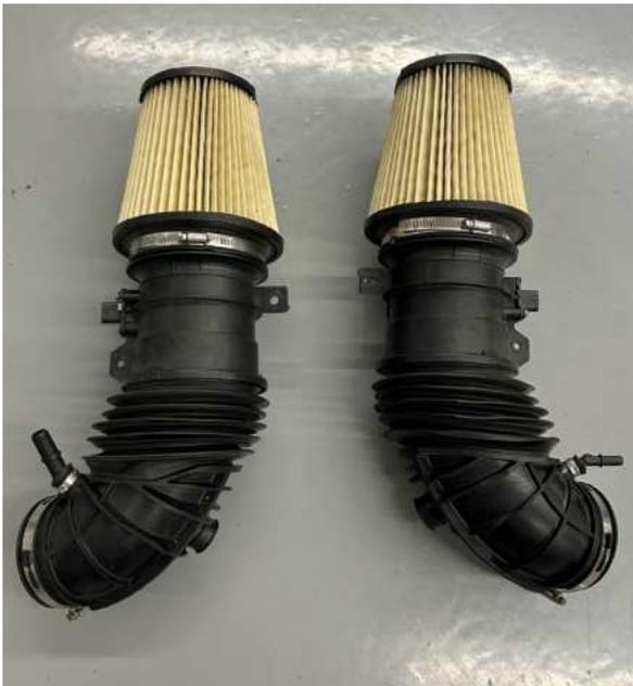
39. Remove the metal J clips from both MAF tubes. They will not be reused.
