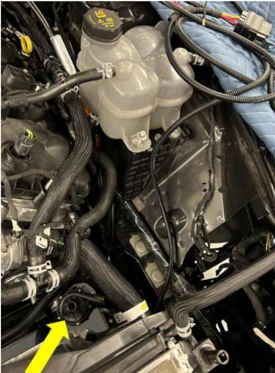
57. Remove the air diverters on each side of the radiator. They will be modified in the next steps. (Trim tool required)
