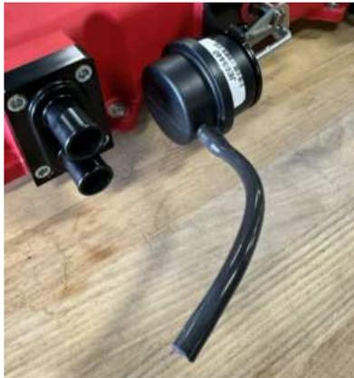
77. From the supercharger assembly, retrieve the 2 fuel rail ports taped to the side in a plastic bag. Install them on the fuel rail holes on both driver and passenger side. Torque to 30 Nm.
