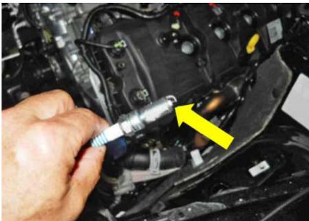
15. Install the supplied spark plugs into all 8 cylinder locations. Torque them to 15 Nm. Reinstall the 7 coils back into the 6 cylinder locations and spark plug boot into the cylinder #3 location. Torque the coil bolts to 10 Nm. Reconnect the electrical connectors to the 8 coils. (5/8 spark plug socket, 8mm socket)
