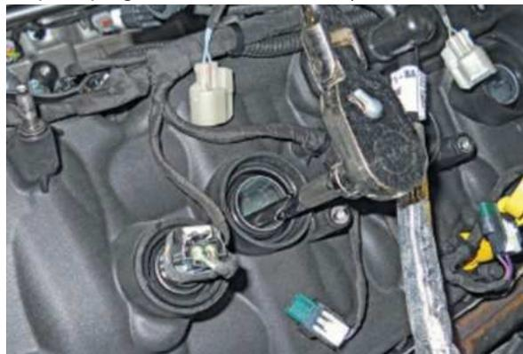
16. Modify the engine degas hose located on the left side (driver side) of the engine as shown. Remove 3/4" inch of hose from the bleeder hose as shown. The cut should be close to the bottom of the word ENG. Reinstall the hose onto the barb and reuse the factory constant tension clamp.
