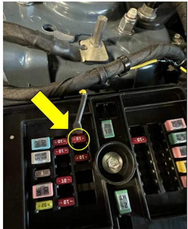
122. Cut a notch in the fuse panel lid as shown. This is to allow the trigger wire to pass thru the fuse panel without getting pinched. Re-install the fuse panel cover onto the fuse box.
