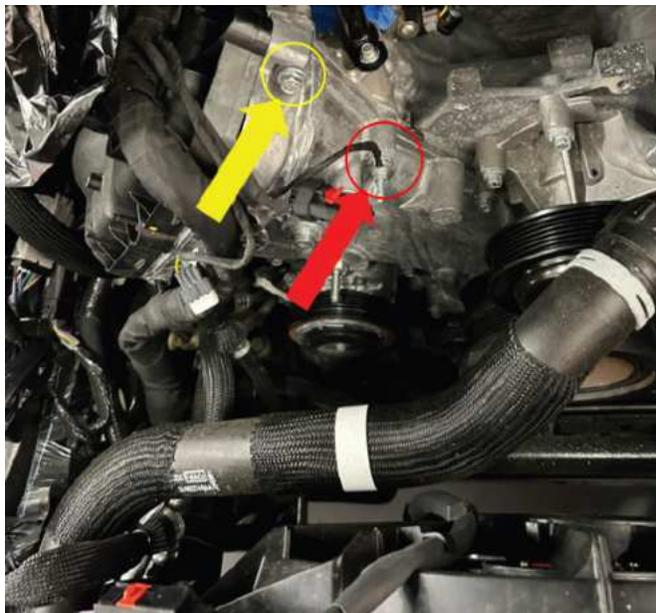
38. Previous step completed with the ground stud moved to new position as shown.
