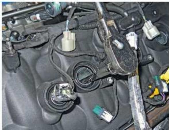
14. Locate the new 8 spark plugs (Item 42, page 10) from hardware kit 31-26-50-029. Verify the gap is between 0.028-0.031" (0.7-0.8 mm). Check to ensure the gap is intact and none are damaged.
