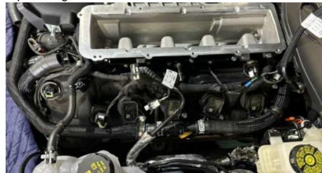
81. Gather the provided 3 bolts M6x75mm (Item 45, page 9) and 7 bolts M6x30mm (Item 44, page 9) (supercharger to cylinder head bolts) from hardware kit 31-26-50-029. Using blue Loctite on the bolts, install and torque them to 10 Nm then to 16 Nm. Follow torque sequence shown.
