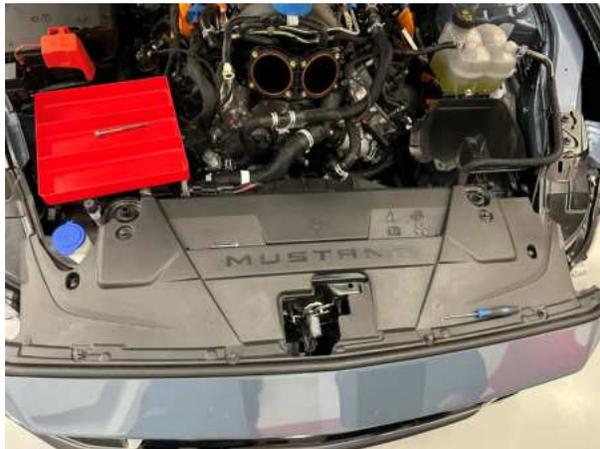
23. Remove the bolt holding the lower left hand (driver side) airbox tray. Remove the lower airbox tray. It will be reinstalled at a later step. (10mm socket)
