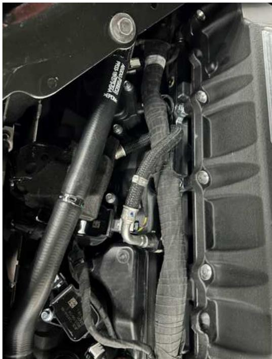
92. Gather the 3/4" quick connect fitting (Item 36, page 6) and hose part number 31-26-50-023F from hose kit 31-26-50-023. This hose will be used for the passenger side heater core return hose.
