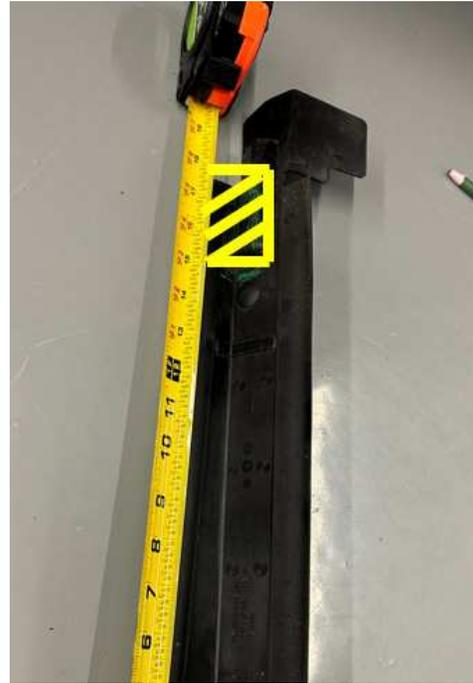
60. Cut the left-hand side (driver side) closeout part on the top section of the part as shown.
