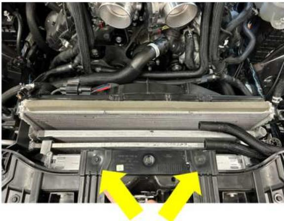
107. Locate the provided degas bottle brackets for both driver and passenger sides (Item 60 and 61, page 10) and degas bottle (Item 27, page 6) Note: If fitted, remove the reservoir cap (Item 28, page 6) from the degas bottle and save for install later.
