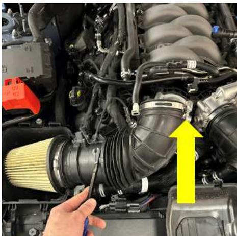
15. Remove the bolt holding the clean air tube to the airbox. (10mm socket.) Remove the clean air tube assembly. Repeat this step on the other side, save all parts for re-use.
