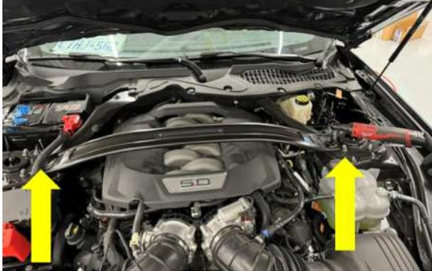
8. Lift up on the engine cover to remove it. It will not be reinstalled.
