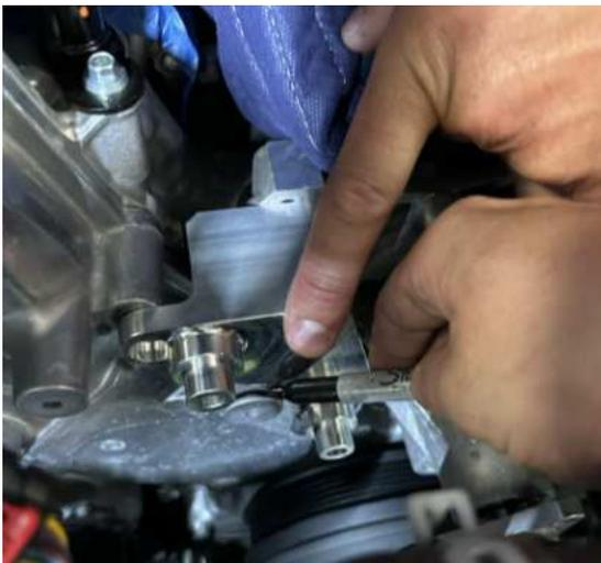
44. Verify the cut from the previous step, it needs to be equal or slightly below the idler bracket when installed. Clean up the debris but keep the engine covered.
