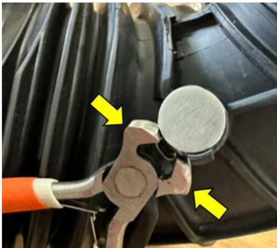
127. Install the modified right-hand side (passenger side) clean air tube assembly from the previous step onto vehicle as shown. Rotate the air filter on the clean air tube so it matches the orientation required on the lower airbox tray as shown. Note: the clean air tube needs to rotate upwards.
