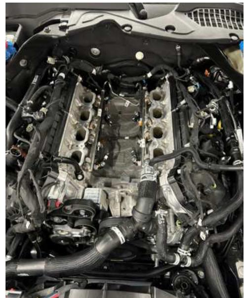
79. With a helper, install the lower supercharger manifold into the engine valley and onto the intake ports with the correct orientation as shown. Route the electrical harness above the SAE quick connect fuel lines.
