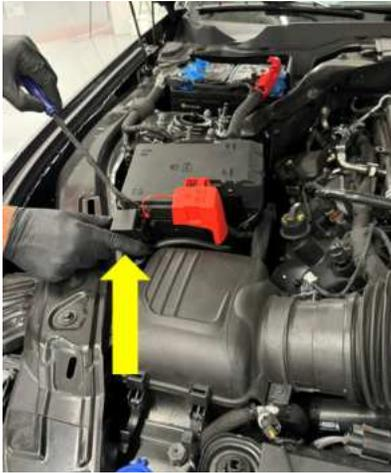
13. Remove the lid from the right-hand (passenger side) airbox. There are 2 latches on the front side.
