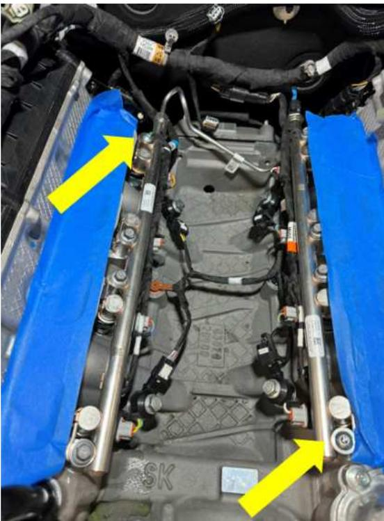
11. Disconnect the electrical connectors for each ignition coil. (7 cylinders, **skip cylinder 3**) Remove the 7 coil mount bolts, keep all hardware for re-use. (8mm socket)
