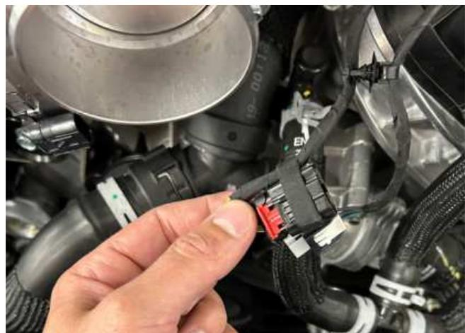
90. Connect the left-hand side (driver side) fuel supply line to the left-hand side (driver side) fuel rail port on the supercharger manifold. Verify it clicks and is engaged onto the fitting.
