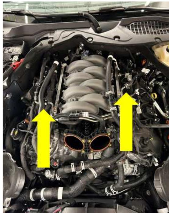
21. Cap all lines that are open to keep debris from getting in. (2 fuel lines and 2 rail fittings)
