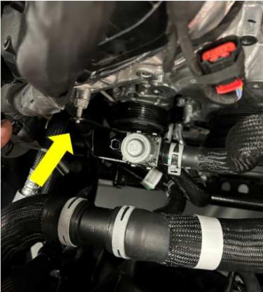
2. Locate the 4 socket head cap bolts M8x60mm (Item 19, page 5). Install the idler bracket (Item 16, page 5) onto the engine. Torque all bolts to 25 Nm. (H6 socket)
