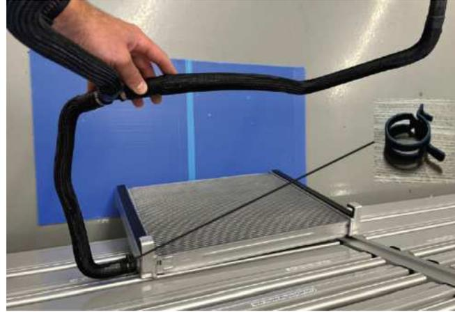
48. Install the LTR to intercooler pump hose onto the LTR (PN: 31-26-50-023C). Use 1 constant tension clamp (orientation shown).
