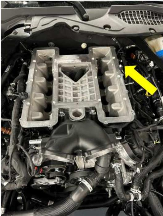
84. Locate the provided supercharger pulley belt PN: K060710 (Item 23, page 5) and loop it around the supercharger pulley (Item 4, page 4) on the lower supercharger manifold. Tighten the 4 M6x16mm supercharger pulley bolts (Item 5, page 4) and use blue Loctite. Note: The bolts will be torqued in step 86.
