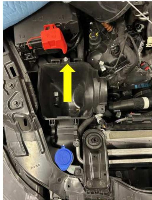
25. Remove the retainer clip from the left-hand side heater hose.
