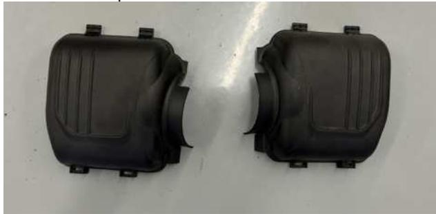
43. Cut  $\frac{3}{4}$ " square off the airbox lids as shown, the corners near the MAF sensor need to be removed. This is to allow clearance for the MAF sensor with the clean air tubes new orientation.
