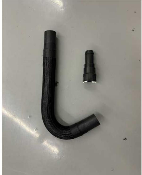
93. Cut 1 inch off of the hose on the side with the bend as shown.
