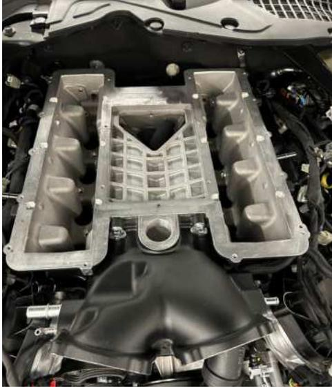
80. Lift each side of the supercharger up and connect the fuel injector electrical connectors (4 per side). Connect the MAP sensor on the back side of the supercharger.
