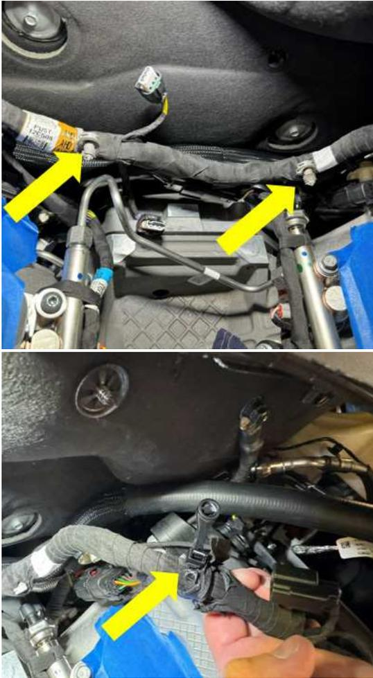
19. Remove the stud shown on the back of the left-hand side (driver side) cylinder head. **Replace the bolt with one of the takeoff MAF to airbox mounting bolts.** (13mm open end wrench, 10mm socket)
