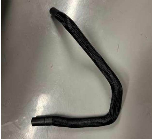
101. Route the hose 31-26-50-023B (from the last step) as shown and install the hose onto the top of the intercooler pump. Use a  $\frac{3}{4}$ " constant tension clamp from hose kit 31-26-50-023 to secure the hose connection as shown.
