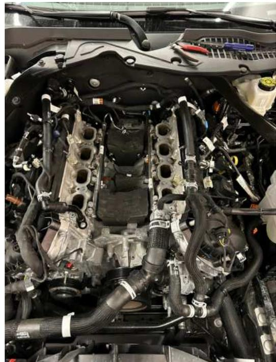
33. Remove the two foam blocks in the valley of the engine. They will not be reused.
