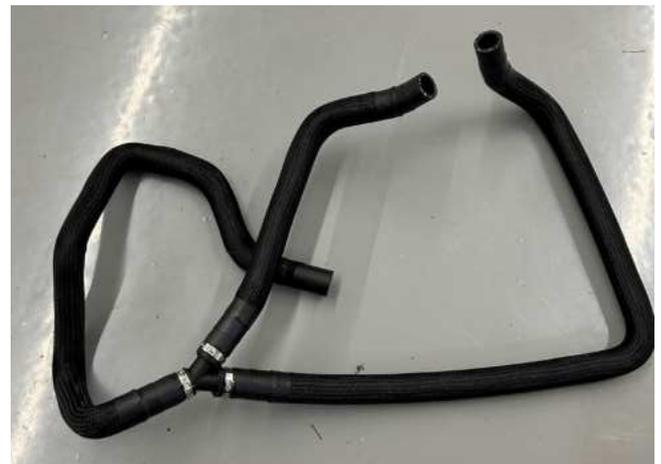
104. Install hose 31-26-50-023A onto the top 2 ports of the supercharger lid. Use 2 power grip clamps (Item 40, page 8) to secure the hose connections to the supercharger assembly. The hose will route around to the left-hand side (driver side) of the radiator core support as shown. (This hose will be connected to the reservoir degas bottle in a later step)
