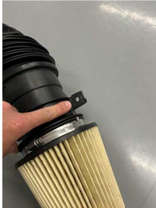
40. Using a grinder or cutting wheel to remove the mounting tab material from both MAF tubes at locations shown below.
