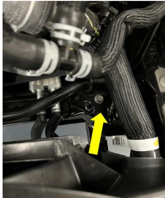
54. Install the provided 15 amp fuse (Item 49, page 8) from hardware kit 31-26-50-027 into the fuse spot on the intercooler pump harness (Item 48, page 8) from the same hardware kit.
