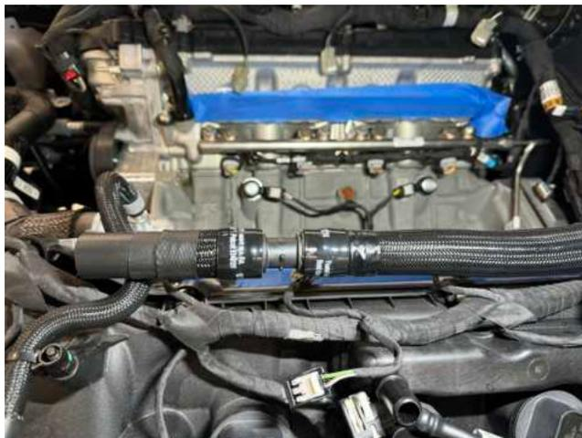
28. For Automatic cars: Located on the front side engine bay, release the constant tension clamps to remove the OEM heater hose off the vehicle as shown. Save clamps for re-use, Discard the hose.
