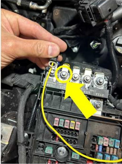
121. Remove the 10 AMP fuse from the fuse box shown (F21 location). Install the intercooler electrical harness fuse jumper onto the fuse and reinstall the fuse.
