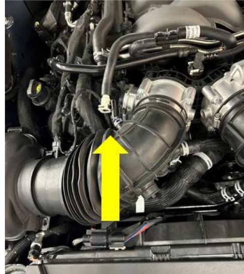
10. Remove the PCV fresh air tube from the left-hand clean air tube. Remove the line from the left-hand cam cover. Save the line, it will be reinstalled.
