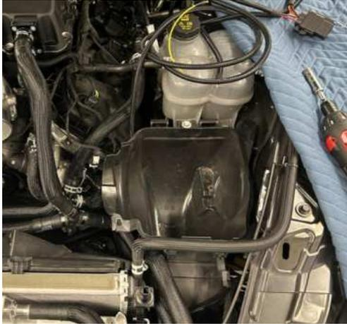
116. Route the intercooler electrical harness relay over to the fuse box area.
