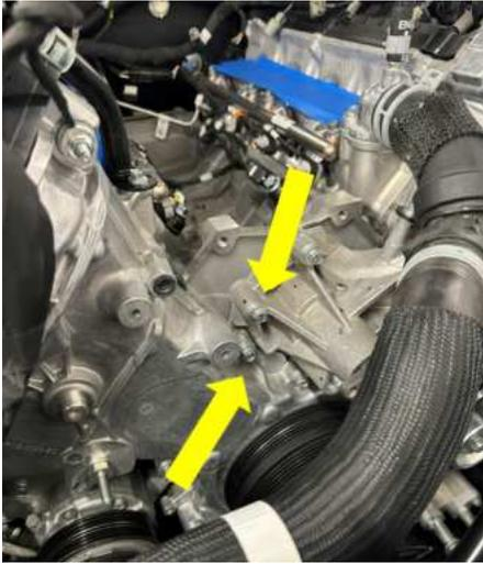
43. Locate and test fit the FEAD bracket (Item# 16, page 5) by holding it up to the front cover to determine cut length shown. The cut must be below the flat surface of the idler bracket mount as shown below.
