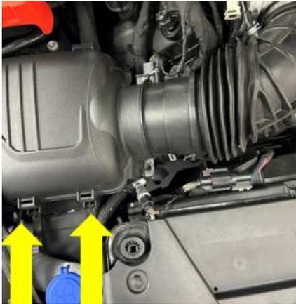
14. Disconnect the MAF harness electrical connector. Use a trim tool to remove the zip tie fir tree from the clean air tube. Loosen the clamp on the throttle body. (7 mm socket) Repeat this step on the other side.
