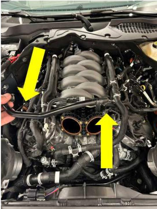
19. Release the quick connect fitting from the right-hand heater hose. Move the heater hose to the side of the engine compartment. It will be modified in another step.
