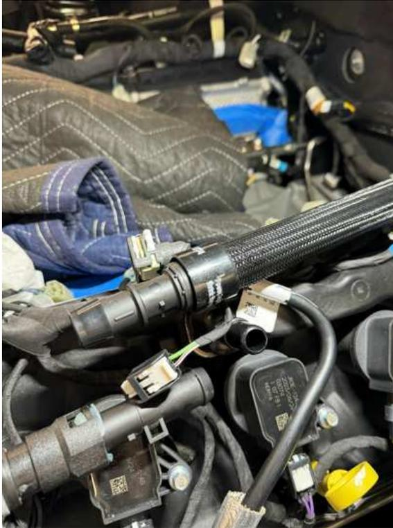
27. For Manual cars only: Take the 4" piece cut from step 22 and install it onto the hose mender with a power grip clamp securing it. Using a heat gun to apply heat to the clamp evenly until it has shrunk around the hose and is shiny.
