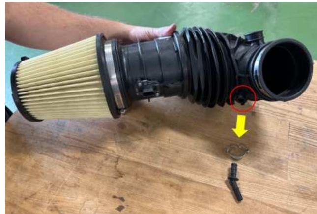
126. Install the new clean air tube plug (Item 47, page 10) found in hardware kit 31-26-50-029 onto the right-hand side (passenger side) clean air tube and clamp (Item 46, page 10) from the same hardware kit using the provided plier tool as shown.
