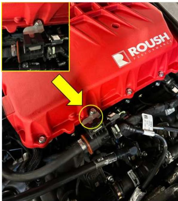
138. Connect the electrical connectors and the fitting from the engine harness to the EVAP solenoid.
