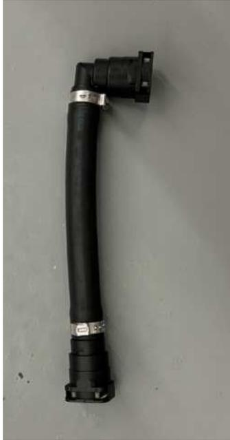
98. Install the PCV hose on the right-hand side (passenger side) cam cover to the right-hand side (passenger side) side port on the supercharger.
