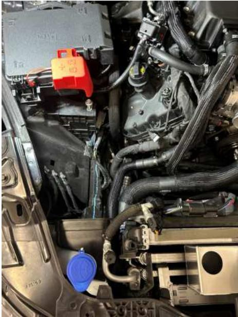
117. Remove the m6 bolt holding the fuse panel in this location. (10mm socket) Reinstall the bolt and mount the relay as shown. The fuse holder can be zip tied to the relay.
