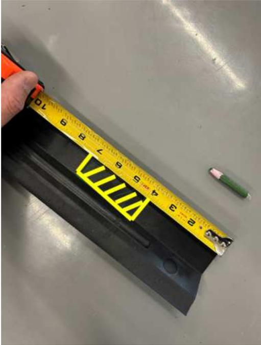
61. Cut the right-hand side (passenger side) closeout part on the location as shown. The mark is 15 inches from the bottom of the part.
