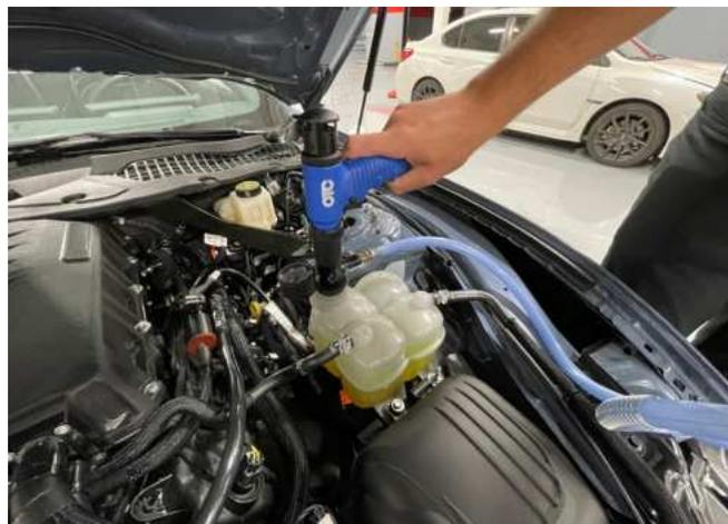
142. Use the same vacuum fill tool and check for leaks on the degas bottle (supercharger intercooler system). If no leaks are found, fill the system using the same tool. **The required fluid level is at 1/8 inch from the top of the bottle as shown.**
