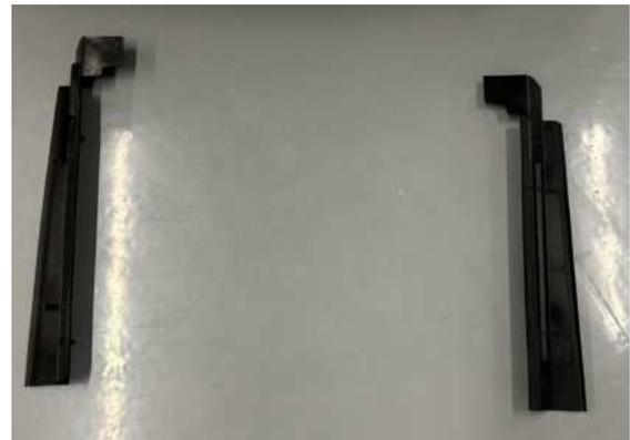
59. Cut the left-hand side (driver side) closeout part on the location as shown. The mark is 4 inches from the bottom of the part.
