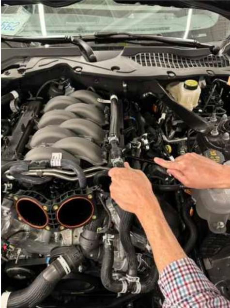
26. Disconnect the quick connector fitting on the left-hand heater hose. Move the hose towards the outside of the engine bay.
