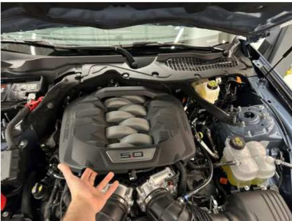
9. Locate the quick connect fitting on the right-hand clean air tube. Squeeze the fittings and pull to remove it.
