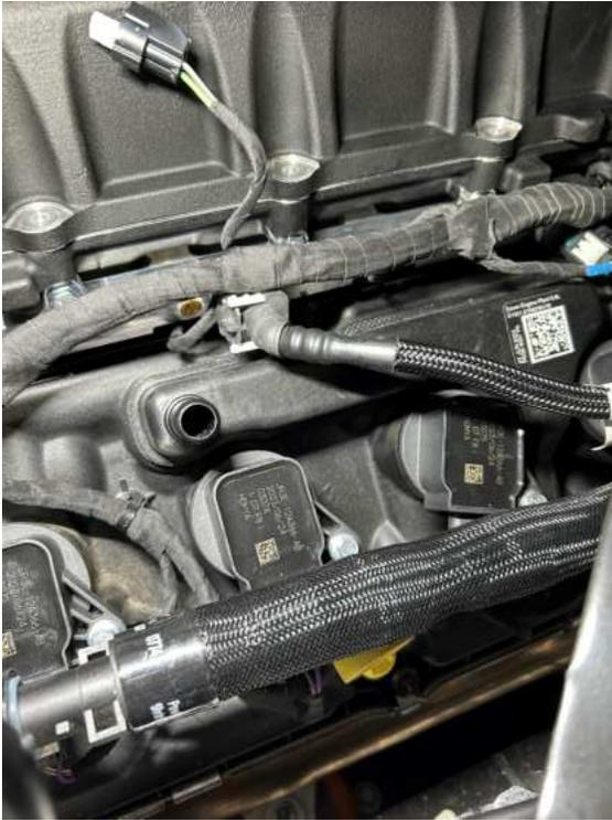
91. Connect the right-hand side (passenger side) fuel supply to the DI pump. Make sure it clicks and is engaged onto the fittings.
