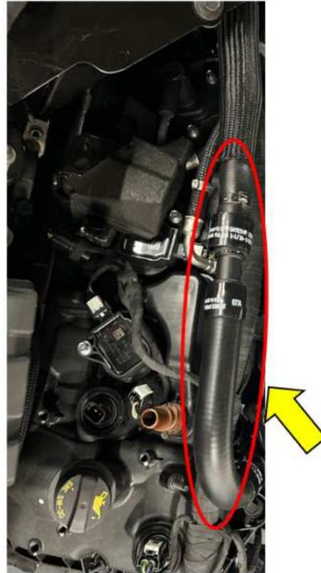
95. **For Automatic cars:** Hold the new heater hose extension line up next to the old heater hose on the right side (driver side) of the engine bay. Cut the heater hose and install the hose mender (Item 36, page 6) to connect the new hose to the end of the old hose.
