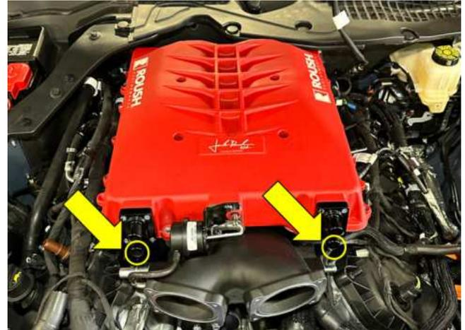
103. Gather the supplied hose 31-26-50-023A from hose kit 31-26-50-023. This will be used to connect the top 2 ports of the supercharger assembly to the reservoir degas bottle.
