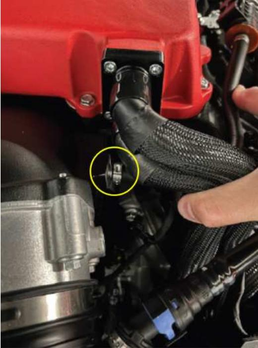
140. Reinstall the takeoff PCV hose from the left-hand camshaft cover to the clean air tube.
