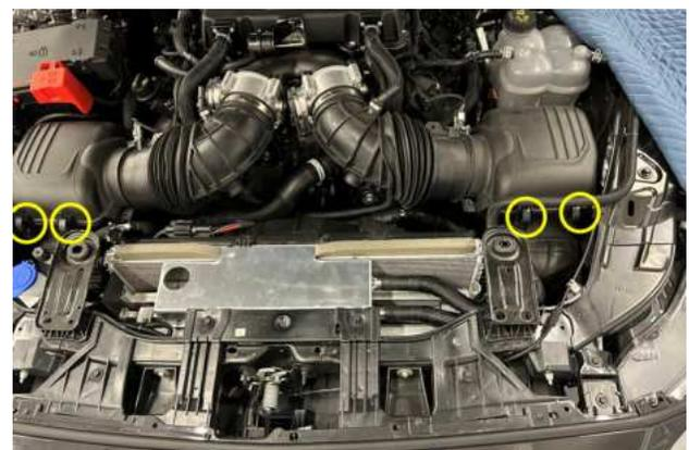
131. Locate the left-hand side (driver side) heater hose mount. Take the grommet off the evap solenoid mount. Note: picture shown below is off the vehicle.
