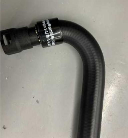
96. Install the provided protective sheaving over the hose section on the right side (driver side) of the engine bay. Use the heat shrink to hold it into place.
