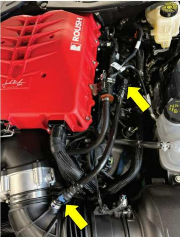
Step 140 Continued: Before installation, using a heat gun to apply heat to the PCV hose evenly and bend the PCV hose straight slightly as shown, this will ease the installation process.
