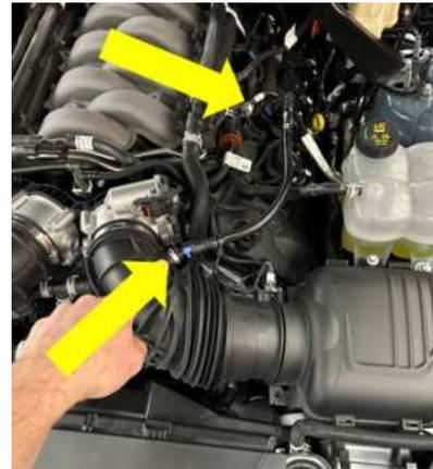
11. Remove the airbox lid from the left-hand clean air tube. There are 2 latches on the front side. Save airbox lid for re-use.
