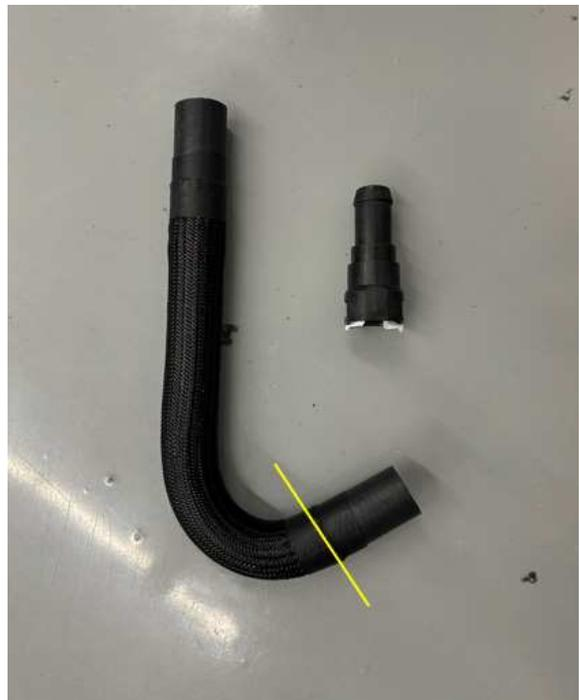
94. Install the quick connect fitting onto the end of the hose from the last step as shown. Using a power grip clamp (Item 40, page 8) to retain the fitting. Using a heat gun apply heat to the clamp evenly until it has shrunk around the hose and is shiny.
