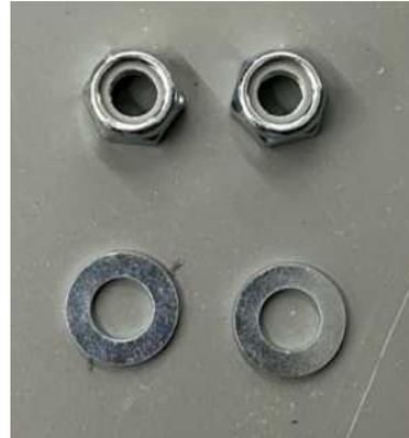
68. Install the washer and lock nut on the bottom 2 mounts for the LTR (washer goes under the lock nut). Install them until they bottom out. Torque to them to 15 Nm.
