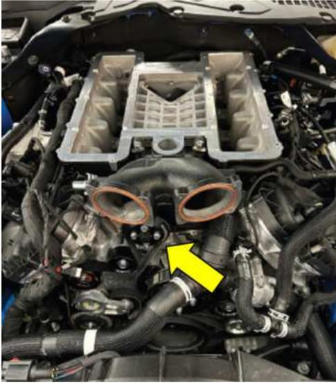
88. Re-install the 2 stock throttle bodies removed from the factory intake manifold onto the supercharger manifold with the correct orientation as shown. Torque the bolts to 12Nm. (8mm socket)
