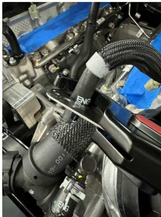
17. On the back side of the engine, remove the harness retention clip from the electrical harness. They will not be reused. (3 locations)
