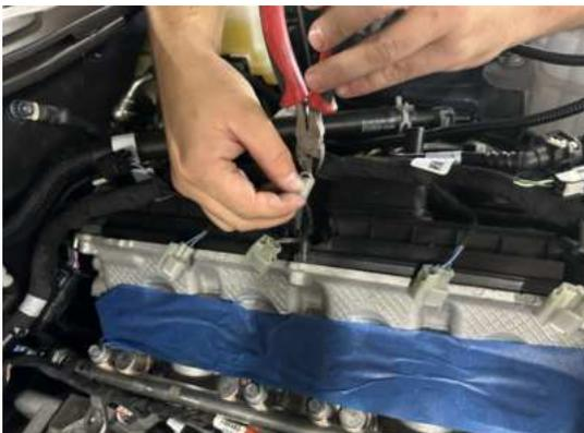
76. Remove the bypass hose from the port on the side of the inlet and lift to remove the supercharger lid.
