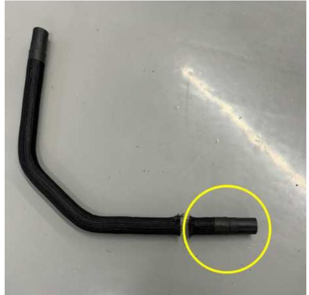
23. Located on the left side (driver side) of the engine bay, Release the constant tension clamp and remove the male quick connect fitting off the OEM heater hose. Save part for re-use.
