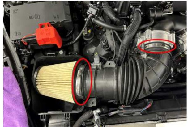
129. Locate and install the left-hand side (driver side) clean air tube assembly. Rotate clean air tube and air filter to the correct orientation as shown. Tighten the air filter to the clean air tube clamp (8mm socket), then tighten the clean air tube to the throttle body clamp (7 mm socket). Torque to 4.1 Nm.
