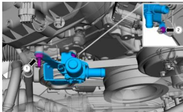
42. Remove the 2 bolts from the water pump at the location show, they will not be reused.
