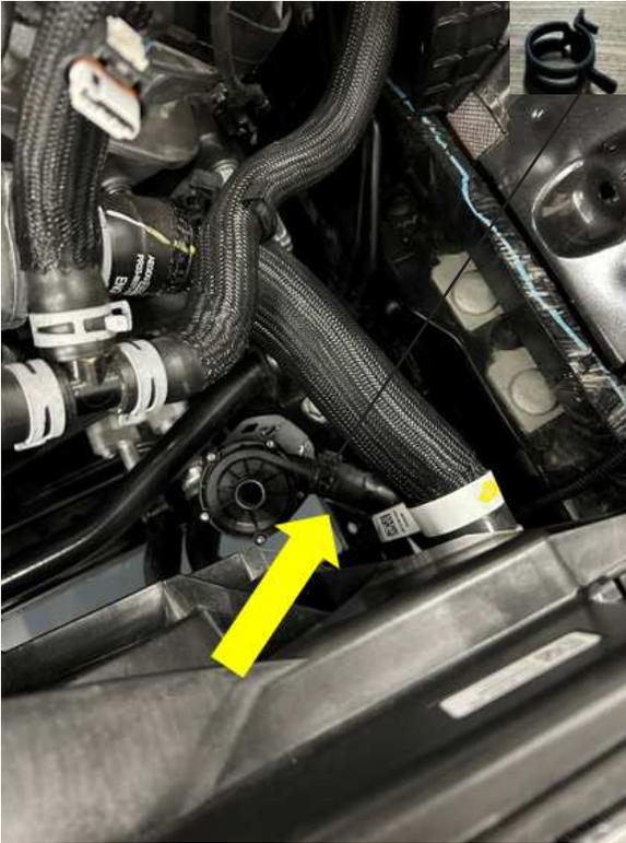
70. Remove the quick release clip located on the right side (passenger side) of the engine if it is still installed on the heater hose hard line shown.
