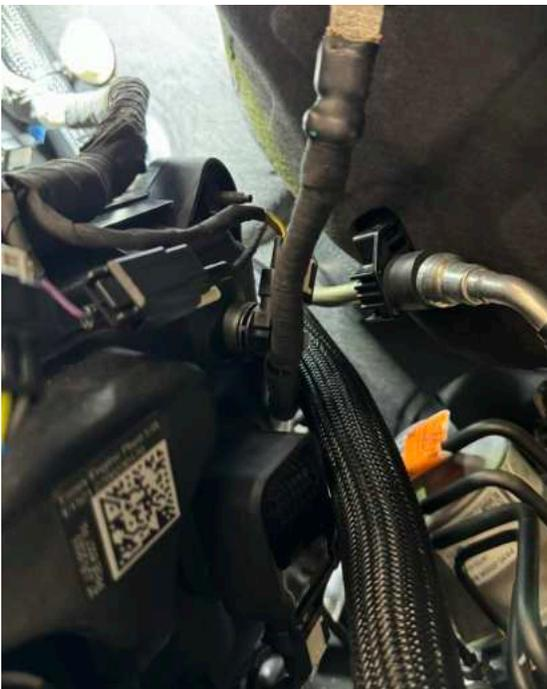
26. For Manual cars only: Install the provided  $\frac{3}{4}$ " hose mender (page 8, Item 39) and power grip clamp (page 8, Item 40) from hardware kit 31-26-50-027 at the end of the OEM heater hose on the left side (driver side) as shown. Using a heat gun to apply heat to the clamp evenly until it has shrunk around the hose and is shiny.
