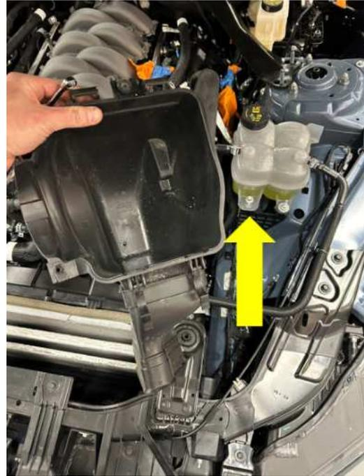
24. Remove the bolt holding the lower right hand (passenger side) airbox tray. Remove the lower airbox tray. It will be reinstalled at a later step. (10 mm socket)
