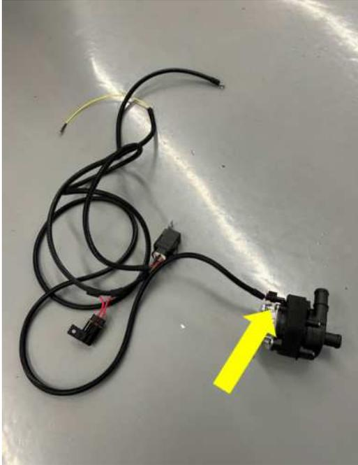
56. Install the intercooler pump into the location on the intercooler pump mounting bracket (from step 53), make sure it is the same orientation shown. Leave the wiring harness to the side of the engine bay.
