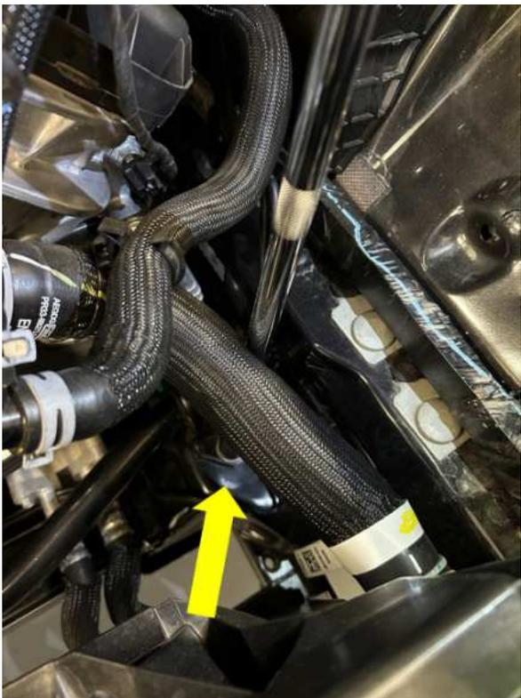
53. Install the intercooler pump bracket and reinstall the sway bar mount bolt as shown. Torque to 110 Nm.
