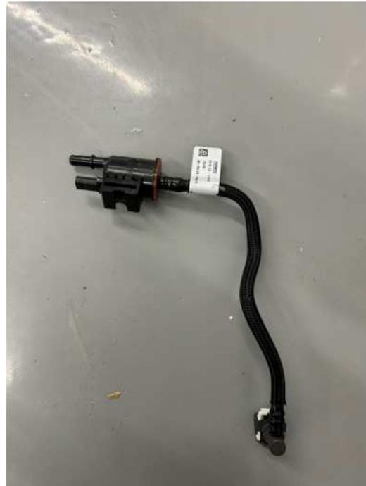
132. Install the EVAP solenoid grommet onto the metal bracket (Item 43, page 10) supplied in hardware kit 31-26-50-029.
