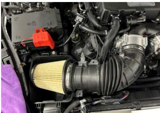
128. Tighten the air filter to the clean air tube clamp (8mm socket), then tighten the clean air tube to the throttle body clamp (7 mm socket). Torque to 4.1 Nm.
