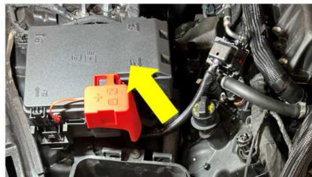
119. Route the intercooler electrical harness power line along the fuse panel and connect the eyelet to the power terminal shown.
