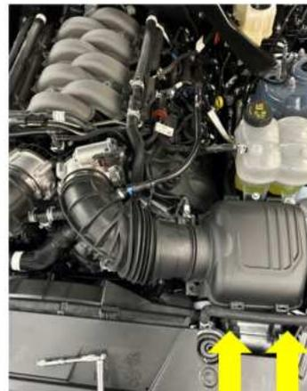
12. Remove the relay from the power distribution block, save relay for re-use. This can be done by releasing the clip with a flat blade screwdriver.
