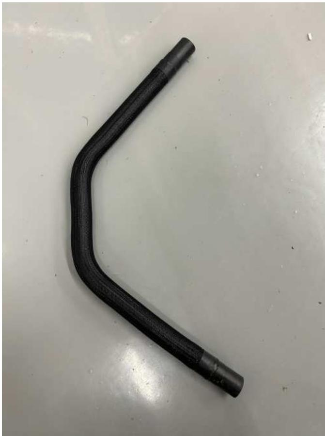
22. **For Manual cars only:** Modify the hose from the last step as shown. Cut 4 inches of hose from the end, keep it for install in a later step. Discard the rest of the hose.
