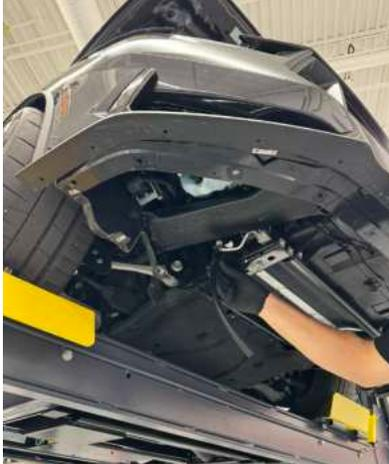
7. Remove the strut tower brace. Locate the 4 mounting nuts. (15mm socket) Reinstall the takeoff bolts (Torque: 41 lb.ft (55 Nm)) . Note: The strut tower will not be reinstalled. Note: Non-Darkhorse or Non-Performance Pack 5.0 Mustangs may not be equipped with the strut tower.
