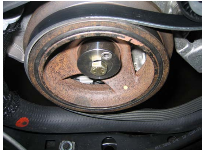
Drill Jig Installed
