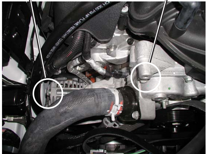
Coolant Reservoir Mounting Locations
