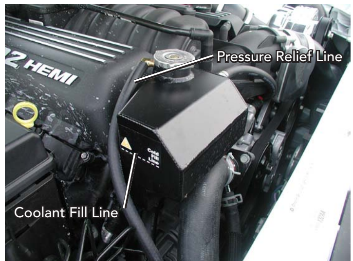
Pressure Relief Line Routing and Fill Line
