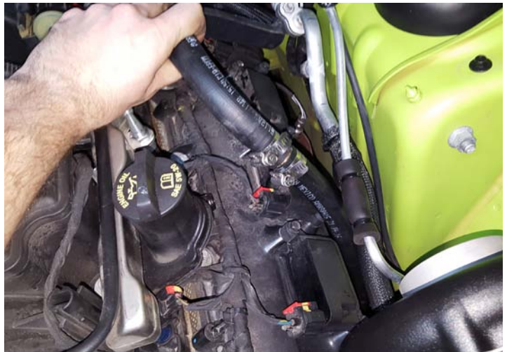
New 3/4" Hose Connected
