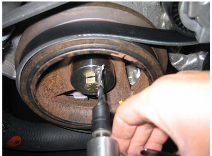
Drilling the Crank
