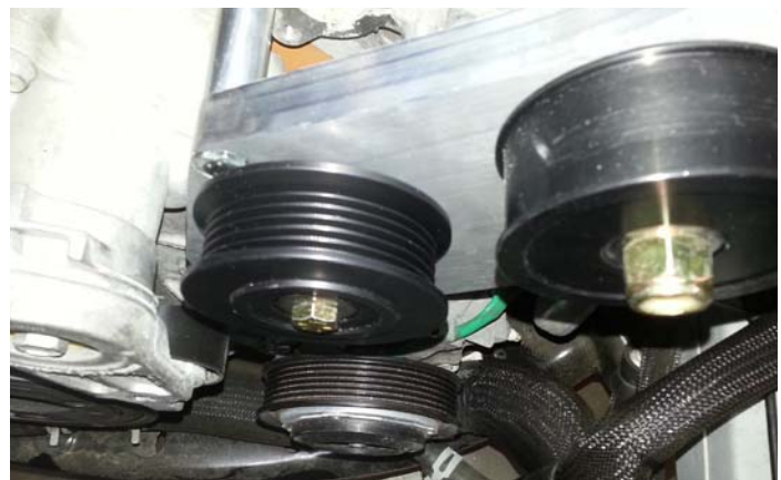
Ribbed Idler Installed
