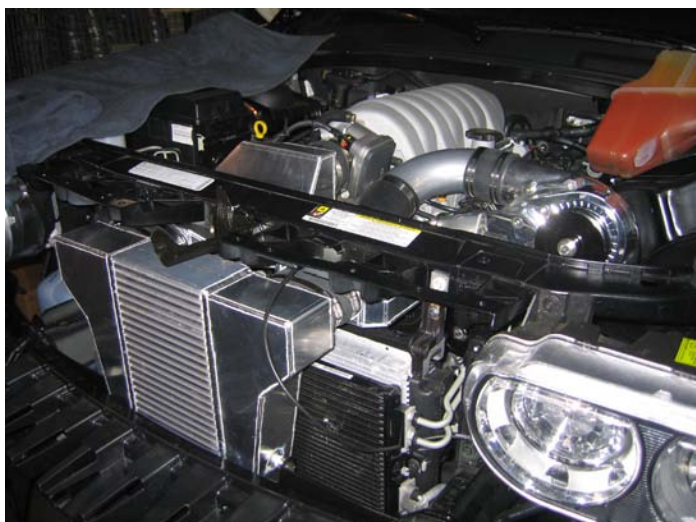
Intercooler and Tubing Installed
