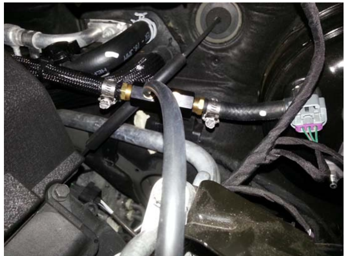
Vacuum Manifold Installed
