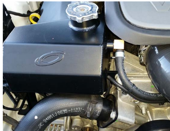
Coolant Hoses Connected
