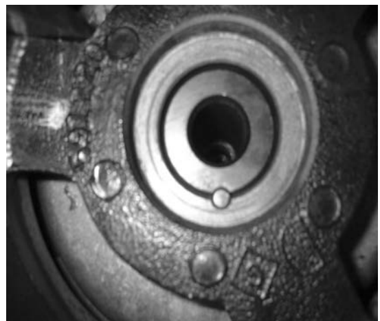
Crank Pulley Pinned to Crankshaft
