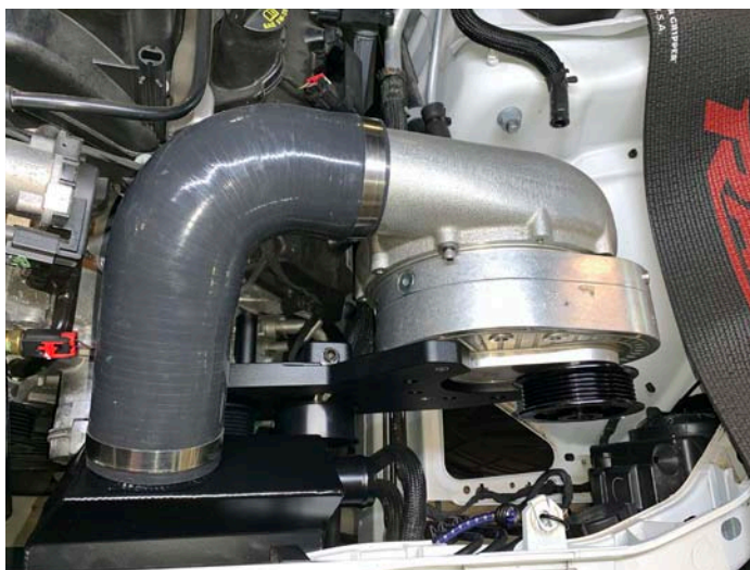
Tube and Reducer Installation
