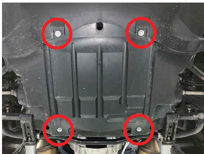
Remove Back Cladding
