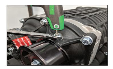
2. Once the locknut is loosened you can back the set screw off.
