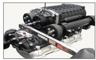
12. Once the idler bolt is torqued hold the set screw in place while you tighten the lock nut.
