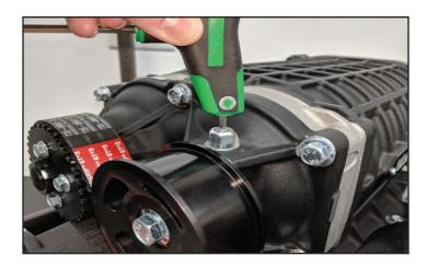
11. Double check the torque for the idler bolt is at 25 ft-lbs once the belt tension is properly set.
