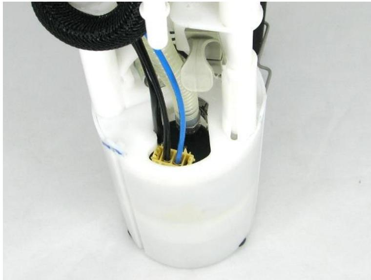
8 – reinstall the assembly into the fuel tank and attach a length of hose to the outlet of the pump assembly allowing it to drain into a fuel safe container and prime the fuel pump assembly
