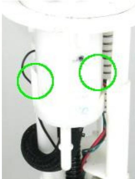
6 – before reinstalling the hat assembly into the center/bucket assembly, push both the 3/8" pump outlet hose and tighten the hose clamp and push on the 1/8" venturi feed hose and crimp the 1/8" permanent clamp in place using dykes or side cutters. Now push hat assembly into the center/bucket assembly and push the pump outlet tube onto the hat assembly
