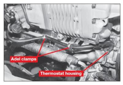
Note: a spare clamp has been provided for Step 21 in case the OE clamp does not fit.
