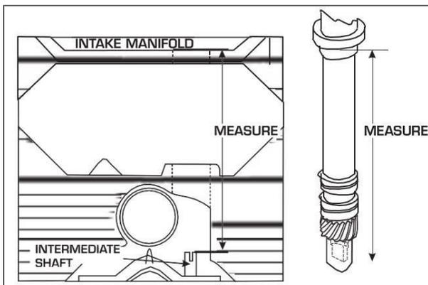
**Figure 15 – Measuring Oil Pump Shaft Overlap**
