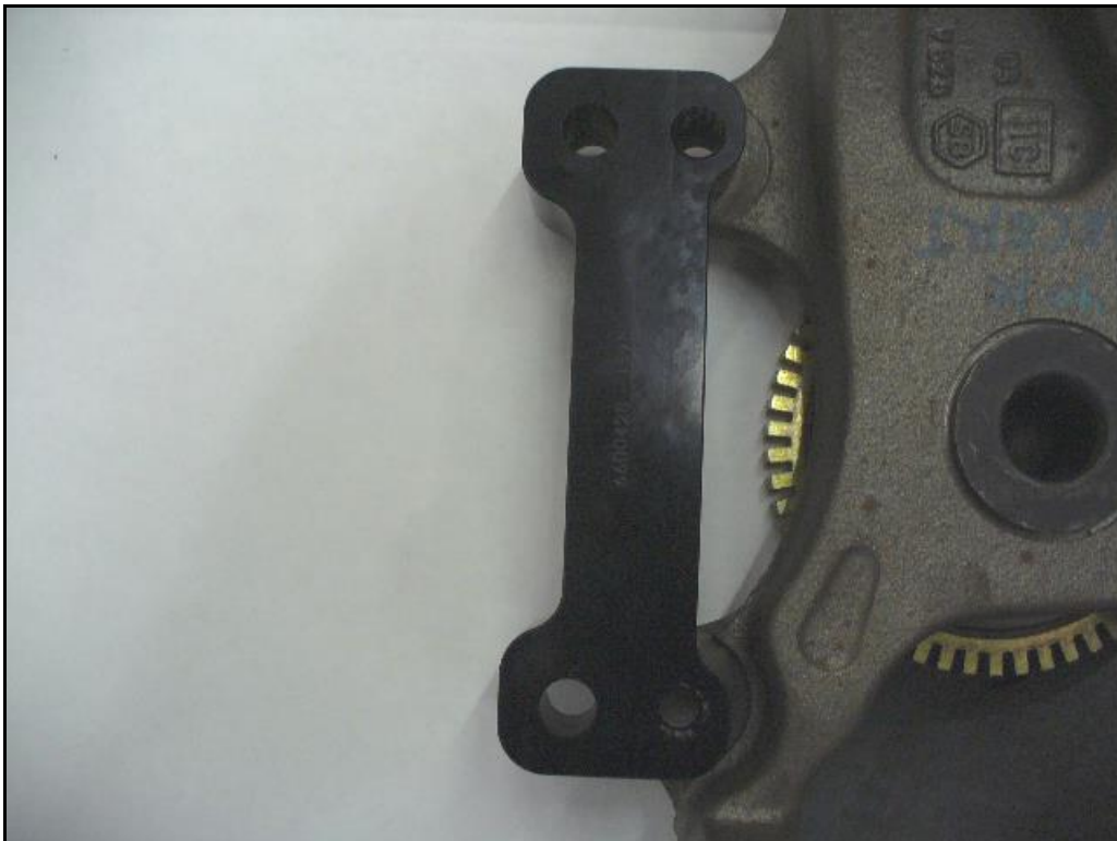
Bracket installed after caliper tabs trimmed.
