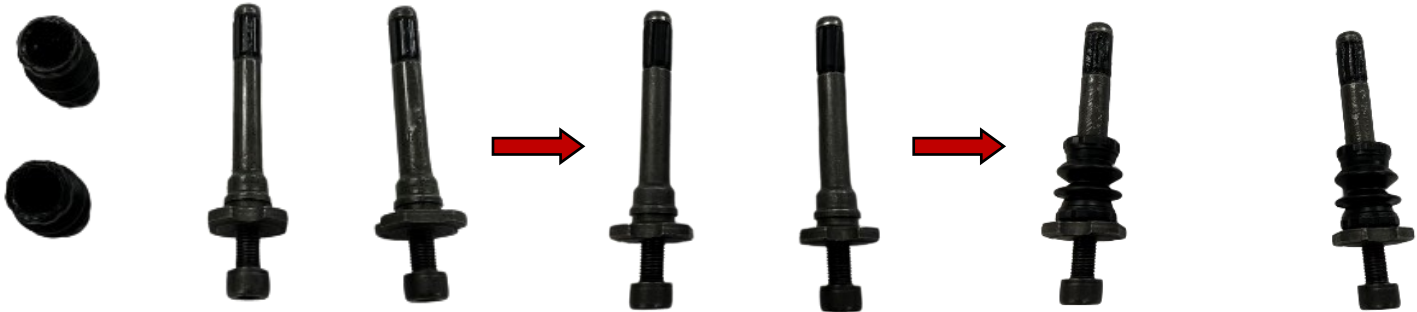
APPLY A THIN, EVEN LAYER OF THE SUPPLIED SILICONE GREASE TO THE PINS AND RE-INSTALL THE RUBBER BOOTS
