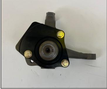
**1.** This installation begins at the point at which the OEM brake components have been removed and the hard lines have been capped to prevent leak down. (Right/Passenger side shown)
