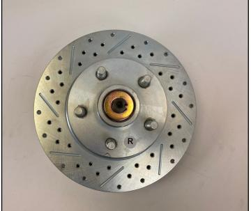
**3.** Next install the correct side rotor. (Right/Passenger side shown). Be carful not to roll or damage the wheel seal when going over the base of the spindle pin.
