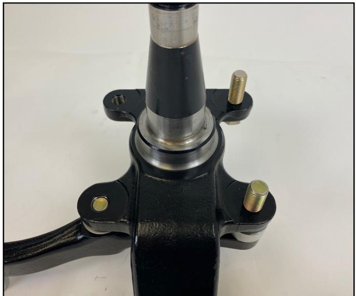
2. Start by threading the supplied 7/16" hex bolts & washers all the way from the inboard side through the spindle as shown. The lower bolt is longer and will go through the steering arm and spacers that came with your spindle.
