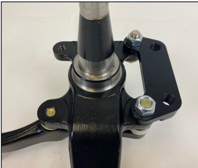
3. Slide the bracket onto the bolts as shown and secure with the supplied 7/16" stover nuts. **Torque these nuts to 75ft lbs.**
