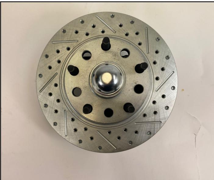
7. Now install the dust cap. Be careful not to dent the dome portion which may lead to interference with the spindle pin or cotter pin.
