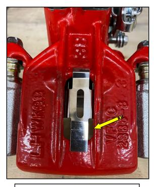
The pad retention spring gets installed into the body of the caliper as shown. Make sure the longer tab is facing the outboard/ front side of the caliper. (Arrow)
