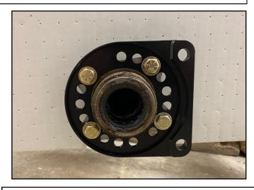
2. Install the correct side Bracket onto the outboard side of the axle using your factory hardware. There are several different clocking options for caliper location. Check your suspension components to make sure the caliper will not interfere with anything. Once verified torque these bolts to the manufacturers specs. (Driver side shown - Bracket is engraved 6710133)
