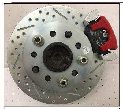
9. View of caliper and rotor installed. Driver side shown. (Left side). Install the hose to the caliper using the supplied banjo bolt and crush washers. Use 1 crush washer on each side of the banjo bolt. Make sure the hose doesn't interfere with any suspension components or the tire/wheel. Torque the banjo bolt to 15 ft lbs.
