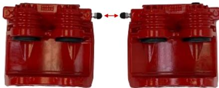
LAY OUT THE CALIPERS, ANCHORS, AND PADS AS SHOWN. THE RIGHT CALIPER AND ANCHOR ARE ON THE RIGHT AND THE LEFT CALIPER AND ANCHOR ARE ON THE LEFT. THE BLEEDER SCREWS SHOULD FACE EACH OTHER. THE CURVED NOTCH IN THE ANCHORS SHOULD FACE EACH OTHER. THE PADS SHOULD BE LAID OUT WITH ONE OF EACH SIDE.
