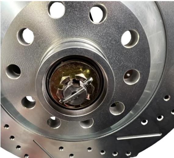
9. Install the provided cotter pin as shown to secure the castle nut.
