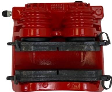
LAY THE CALIPER WITH THE CORRESPONDING ANCHOR AS SHOWN. (PADS MAY OR MAY NOT HAVE WEAR INDICATORS ON BOTH INSIDE AND OUTSIDE PAD)
