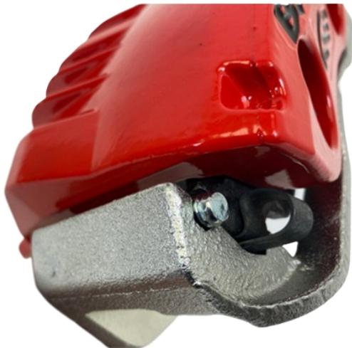
**PUSH THE PIN THROUGH THE OUTSIDE GROOVE BETWEEN THE ANCHOR AND PAD.**
