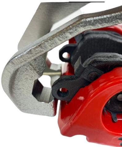
HOOK THE CURVED INSIDE NOTCH ON THE ANCHOR AROUND THE PADS AS SHOWN. (PADS MAY OR MAY NOT HAVE WEAR INDICATORS ON BOTH INSIDE AND OUTSIDE PAD)
