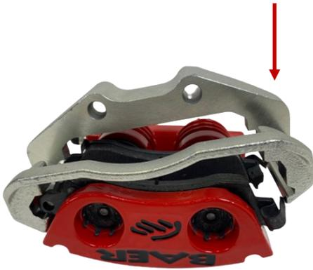
**PRESS THE ANCHOR DOWN INTO THE 'S' CLIPS INSTALLED IN THE CALIPER. YOU MAY HAVE TO COMPRESS THE 'S' CLIPS TO PRESS THE ANCHOR DOWN.**
