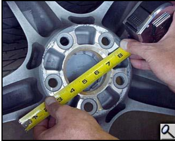
Figure 2: Inside diameter measurements
