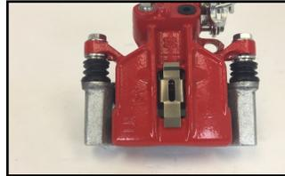
2. Install each pad abutment onto the 'ears' of the caliper. The abutment should face away from the friction surface. There is a small tab that locks into place once installed correctly.
