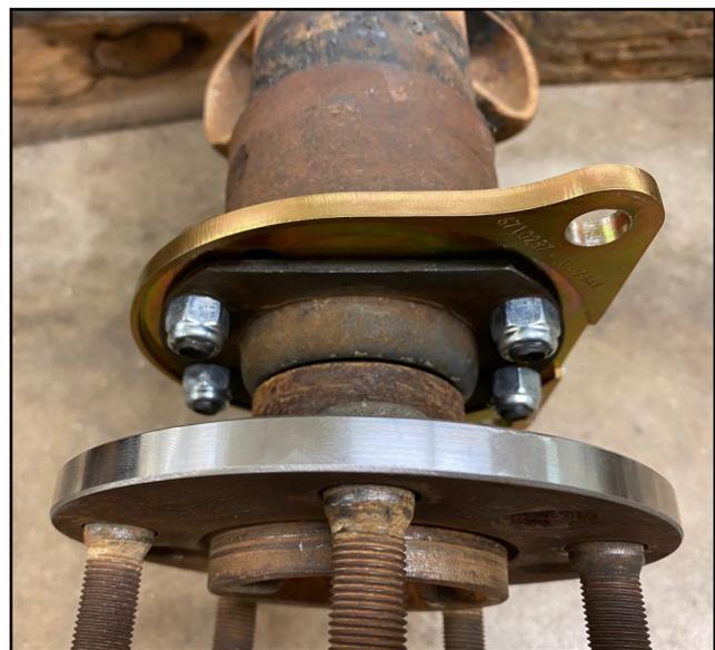
4. Next, line up the bearing retainer on top of the Baer bracket and secure with your factory nuts. (**Axle flange diameter not to exceed 6.125"**)
