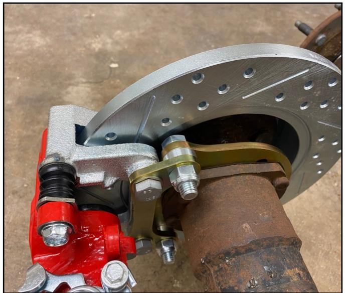
9. Inboard view of the caliper installed. Now that everything is verified, remove the caliper and refer to the next page for pad install instructions.
