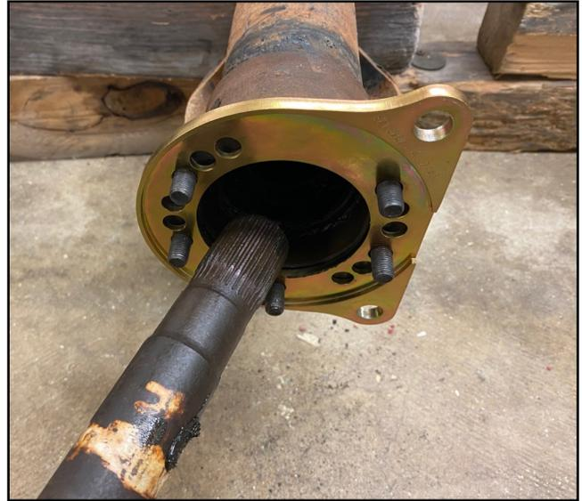
2. Install the base steel bracket onto the 5 studs and set in your desired position as shown. The machined side faces outboard. You can clock the bracket for several positions. (Left rear shown) Do not tighten yet.
