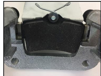
3. Install the pad retention spring into the body of the caliper. From the inside of the caliper body, insert the long tab into the opening and slide it down until the small bent tab clears the piston. Now push the bent tab into the slot and slide it back until it locks onto the ridge on the body as shown.
