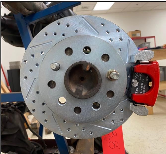
7. Now install the correct side caliper (bleeder pointing up) and secure with the supplied 12mm hex bolts and washers. Check for any clearance issue between the caliper body and the rotor. If all is good torque the bolts to 85ft lbs.
