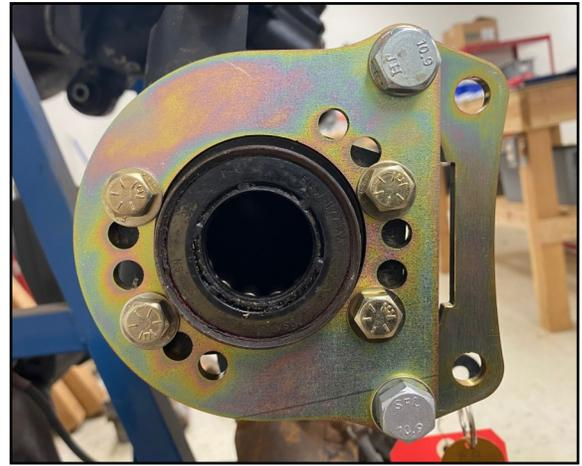
1. Install the base steel bracket using the factory bolts in your desired position using the factory hardware. You can clock the bracket in several positions. Check for any clearance issues with suspension components. (Driver side/Left rear shown) Torque the factory bolts to the manufacturers specs.
