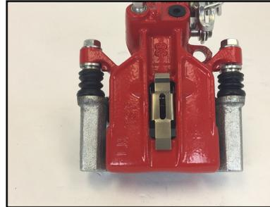
2. Install each pad abutment onto the 'ears' of the caliper. The abutment should face away from the friction surface. There is a small tab that locks into place once installed correctly.
