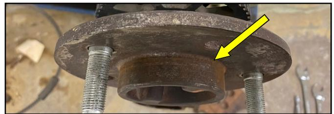
3. Inboard photo showing the intermediate bracket and the location of the spacers. The spacers go in-between the base bracket and intermediate brackets. (See photo)
