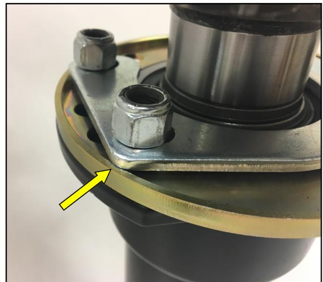
5. Some bearing retainers (Stock and aftermarket) may need to be slightly trimmed to fit inside the relief on the bracket. Grind the retainer minimally to fit. Verify the retainer is sitting flush and torque the 3/8" nuts to 35ft lbs.
