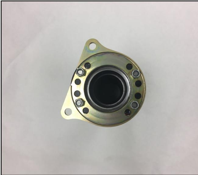
2. Install the base steel bracket in your desired position. You can clock the bracket for several positions. (Right rear shown) Do not tighten yet.
