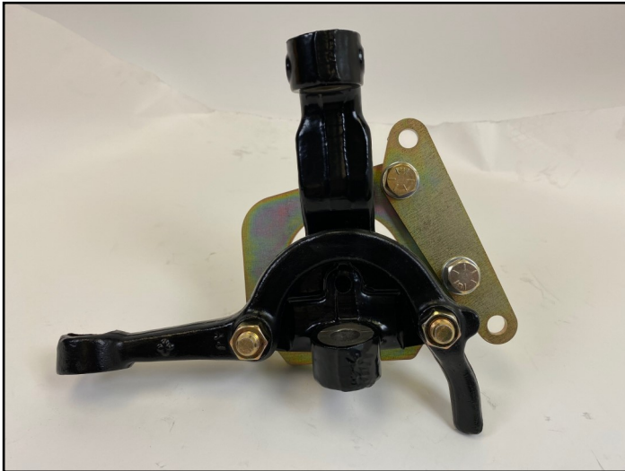
5. Inboard view of intermediate bracket. The long taper pins downward.
