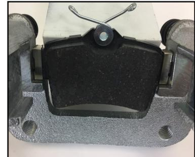
3. Install the pad retention spring into the body of the caliper. From the inside of the caliper body, insert the long tab into the opening and slide it down until the small bent tab clears the piston. Now push the bent tab into the slot and slide it back until it locks onto the ridge on the body as shown.
