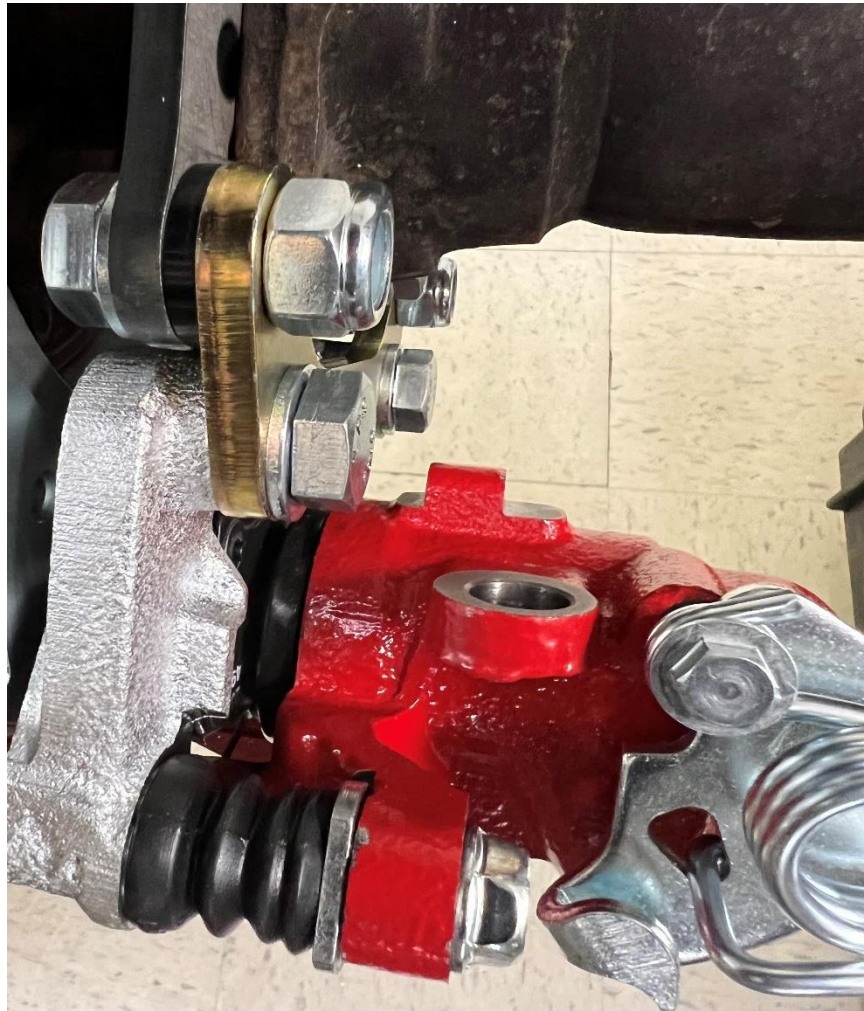
Figure 5. Caliper installed (Inboard View)
