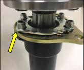
**5**. Next re-install the axle, c-clip, pin, retaining bolt and cover. Now is a good time to check your wheel seal for wear. Replace if necessary. If all is good, torque the differential cover to the manufacturers specs.
