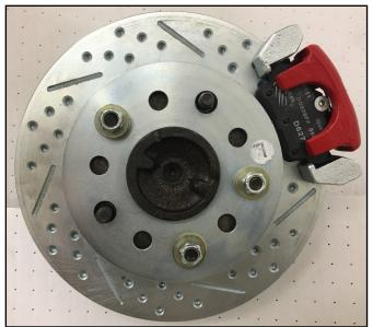
**10.** View of caliper and rotor installed. Driver side shown. (Left side). Install the hose using the supplied banjo bolts and crush washers. Install 1 crush washer on each side of the banjo bolt. Make sure the hose does not interfere with any suspension components or the wheel/tire. Torque banjo to 15ft lbs.
