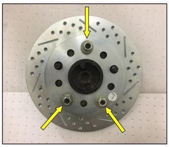
**7.** Now install the correct side rotor and secure with 3 lug nuts. Double check here to make sure the rotor is sitting flat against the axle. (Drivers side shown)
