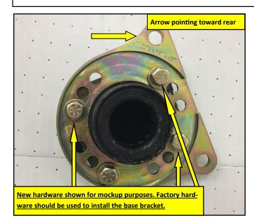
Install the correct side base steel bracket (Engraved 6710278) in the configuration of your choosing. <u>Use your</u> factory hardware to install the base bracket. Torque 3/8" bolts to 33ft lbs. (Left rear shown in trailing position)
