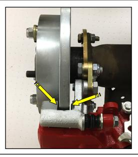
**9.** Double Check that the caliper anchor does not come in contact with the rotor. Once verified, Torque the 12mm hex bolts to 85ft lbs.
