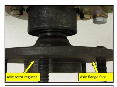
**6.** View of base and intermediate brackets installed along with the axle. Make sure you clean off the axle rotor register and axle flange face to ensure the rotor will sit flat against the axle.
