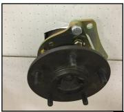
\*With a BOA design you will install the bearing retainer (not included) on top of the steel bracket. Slightly modifying the bearing retainer may be necessary.
