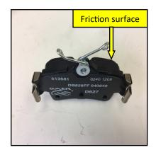
3. Install the pads into the anchor. Put the pad into rotor pathway of the anchor and gently slide the pad and abutments into the inboard side of the anchor. You will be compressing the spring on the side of the abutment as you slide the pad into place. This is a tight fit. Once complete you can do the same for the outboard pad.
