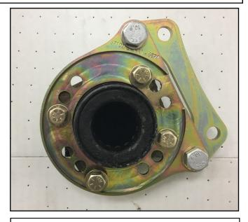
**3.** Install the intermediate steel bracket to the inboard side of the base steel bracket as shown using the supplied 12x30 hex bolts. <u>Make sure the 12mm nylock nuts are installed inboard.</u> Torque the nylock nuts to 85ft lbs
