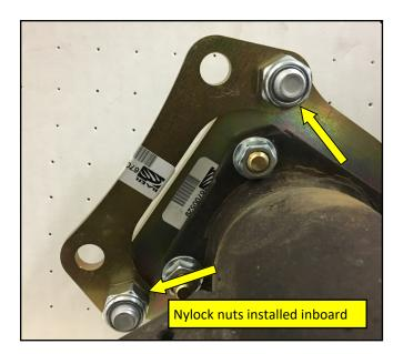
**4**. Inboard view of the intermediate bracket with the 12mm nylock nuts installed inboard.
