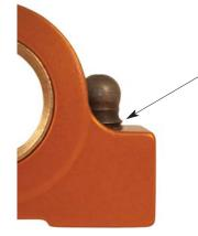
The rocker adjusters are a 7/16-20 screw with a 3/8 ball. You have to use pushrods with a 3/8 cup end. When setting pushrod length have no more than 2 and no less then 0 threads showing on the bottom side of the rocker, between the ball and rocker body. This is to make sure the pushrod contact point and rocker geometry are correct.
