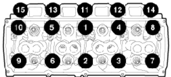
Cylinder head bolt sequence:
