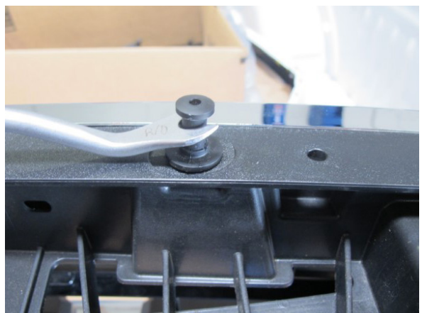
Fig. 1-X: Remove grill plastic fasteners
