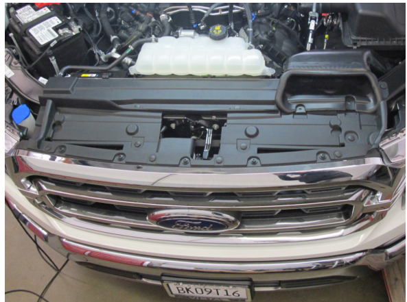
Fig. 9-H: Reinstall radiator support cover
