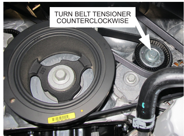
Fig. 1-E: Remove OEM serpentine belt
