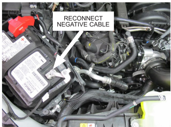
Fig. 9-I: Reconnect negative battery cable
