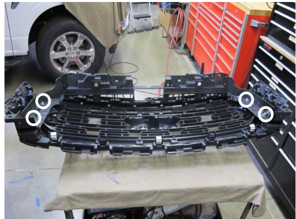
Fig. 2-E: Reattach shutter housing to grill
