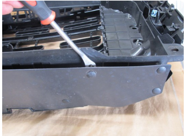
Fig. 1-V: Remove grill lower flap
