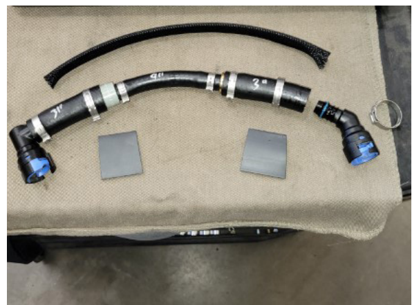
Fig. 2-O: Assemble the new PCV assembly
