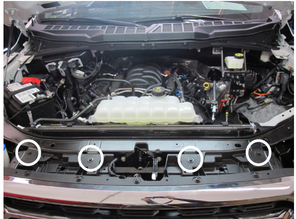
Fig. 1-P: Remove upper grill screws
