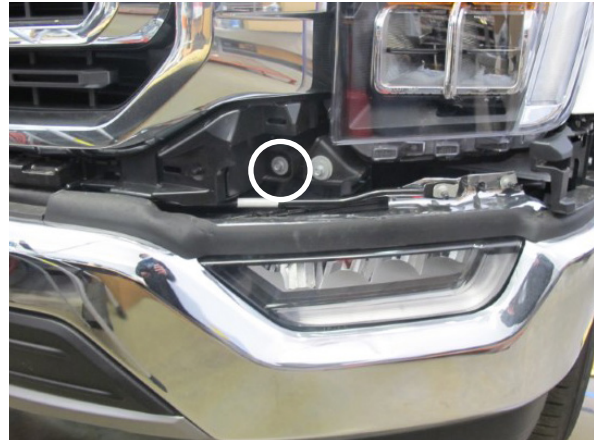
Fig. 1-S: Remove grill lower screws
