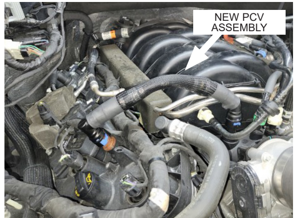
Fig. 2-P: Install new PCV assembly
