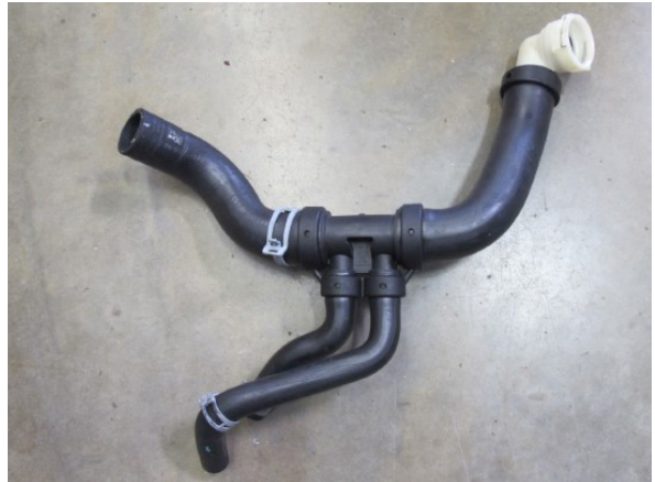
Fig. 1-G: Remove coolant hose assembly
