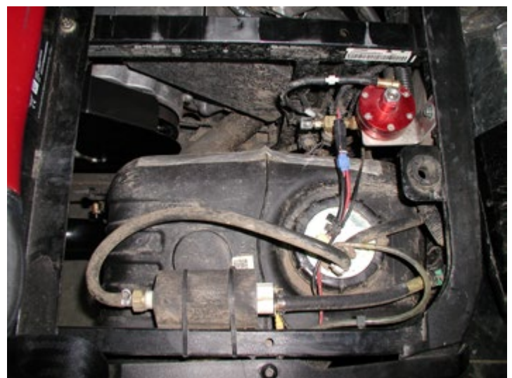
Fuel System Installed
