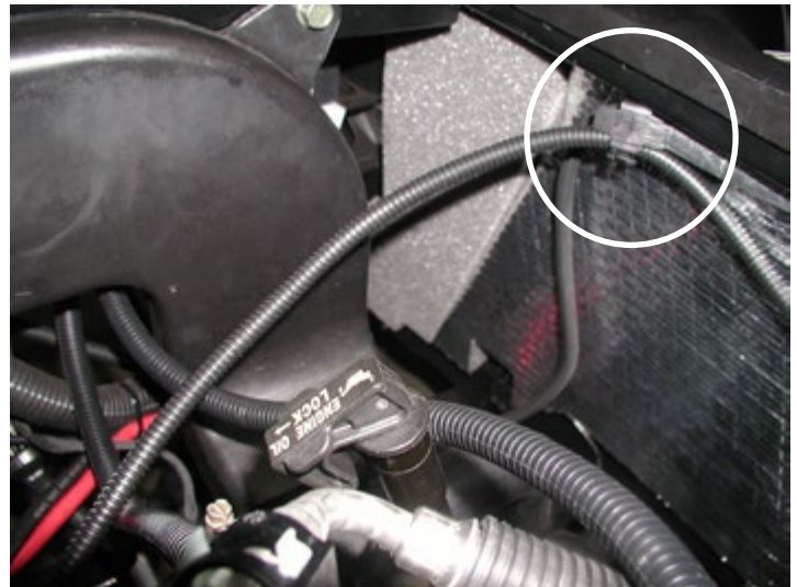
Extension Wire Routing
