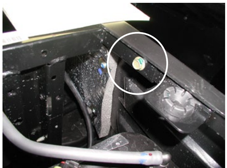
Remove Bolt from Frame
