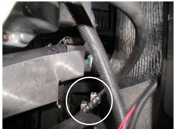
Attach Hose Extension to Factory Hose
