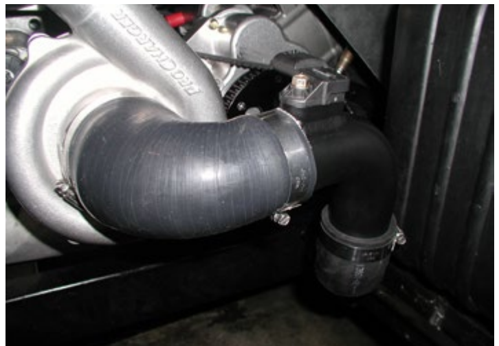
Install Blower Inlet Tube #297
