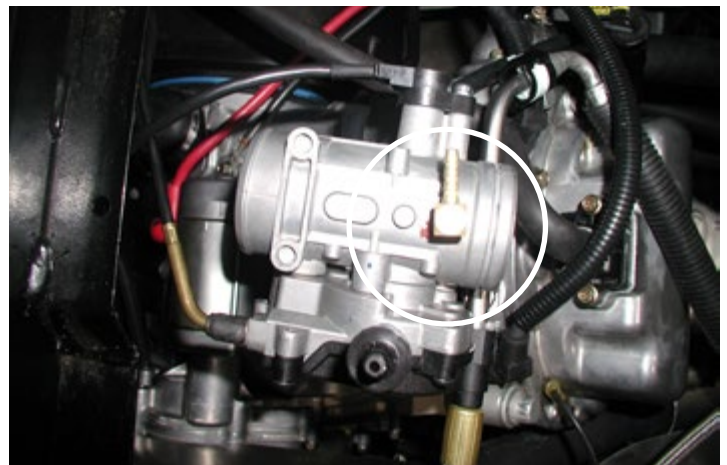
Install Vacuum Fitting
