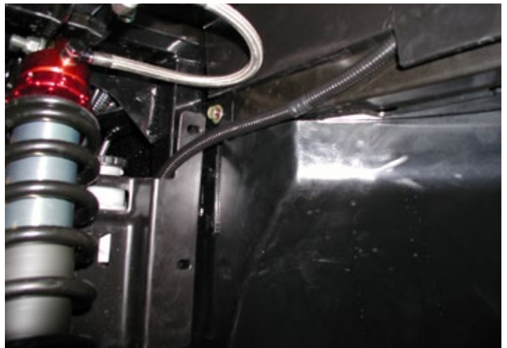
Driver's Wheel Well Wiring Routing
