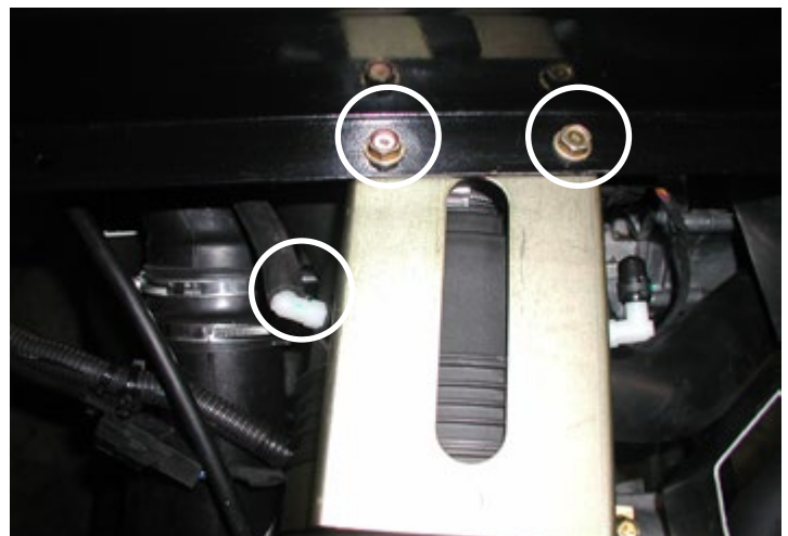
Remove Air Filter Box
