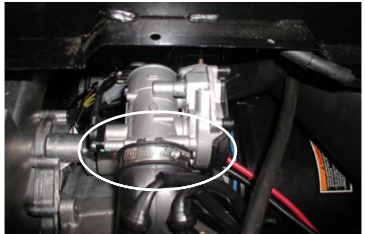
Remove Throttle Body
