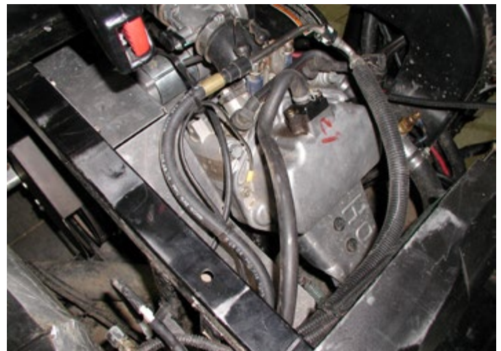
Vacuum Line and Wiring Routing
