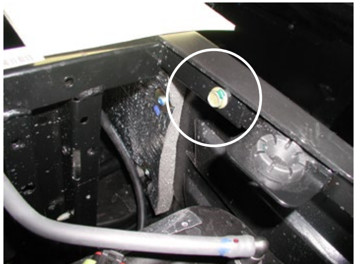
Remove Bolt from Frame
