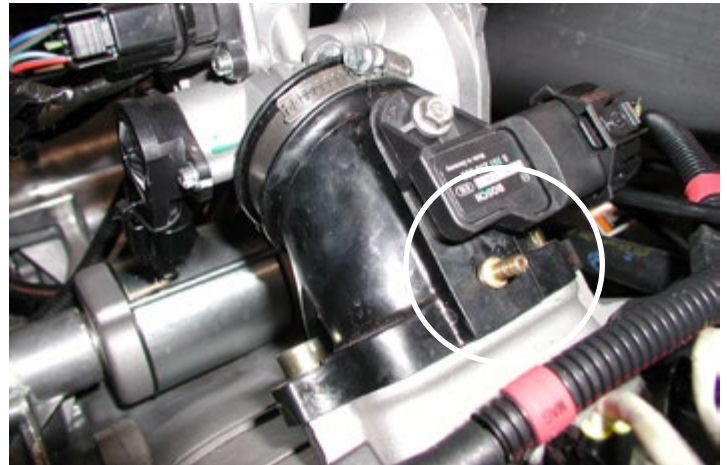
Install Vacuum Fitting
