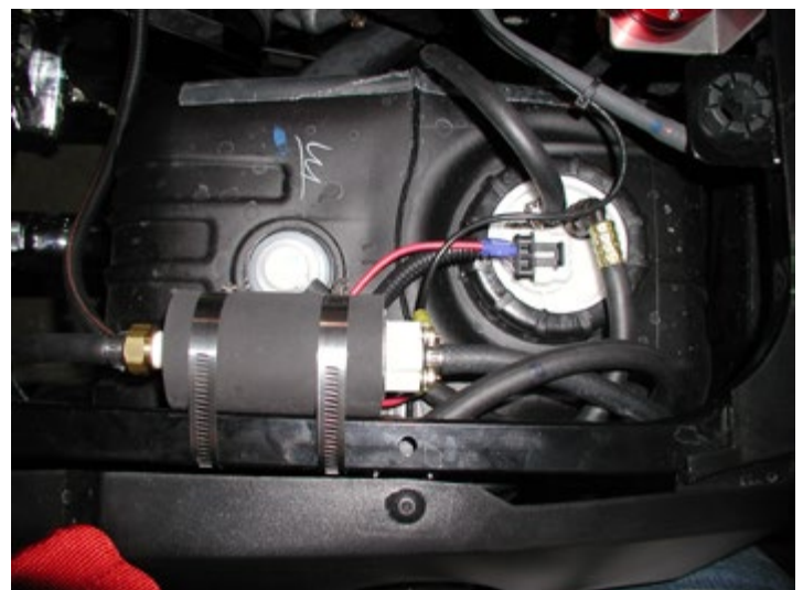
Fuel System Installed
