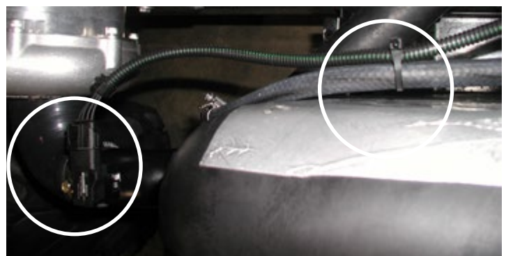
Connect Extension Harness to T-BAP Sensor
