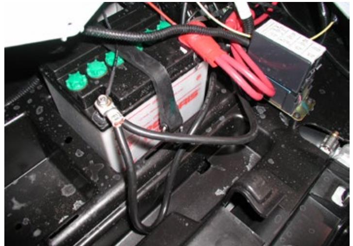
Remove Fuel Pump Fuse, Purge Fuel System then Disconnect Battery
