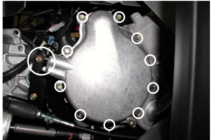
Disconnect CPS & Remove Flywheel Cover
