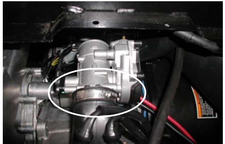
Remove Throttle Body
