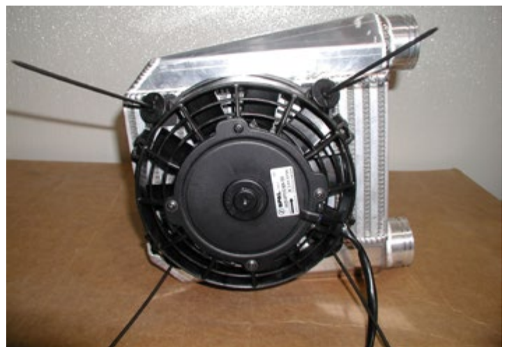
Mount Intercooler Fan & Install Retainers
