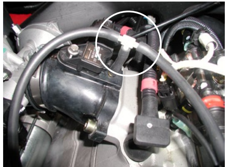
Install Barb T-Fitting into Vacuum Line
