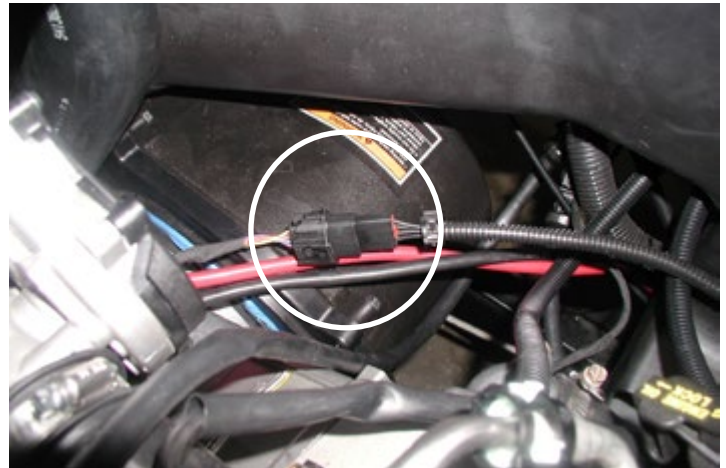
Connect Extension Harness to Factory Harness
