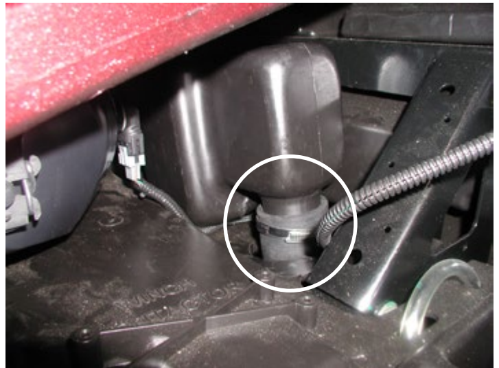
Remove Air Intake Box
