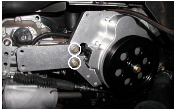
Install Bracket Mount
