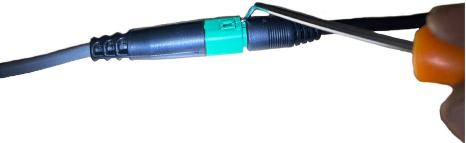
**STEP 3** - Pull the connector apart while holding the clip out.
