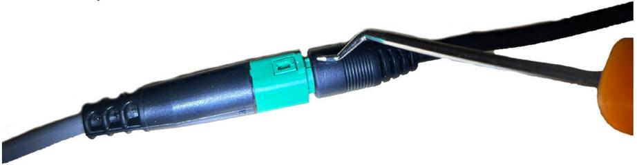
**STEP 2** - Carefully insert the pick tool tip under the connector, and push the locking clip upward/outward to release the connector.
