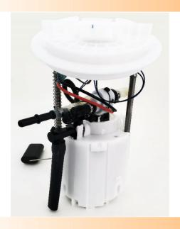
The DW400 Hemi Module is a complete drop in replacement for the OE unit. The module incorporates the DW400 pump which out flows the OE module by 50%. This module also integrates seamlessly with the OE wiring harness and fuel system. The module also utilizes a venturi fed surge bucket for consistent fueling at low tank levels and high G conditions.
