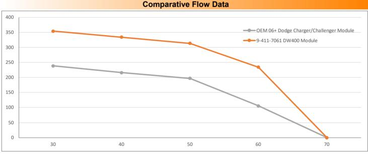
\*Note: Flow testing includes OEM filter and regulator module.
