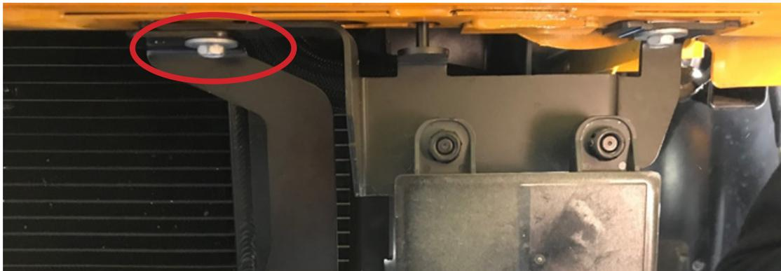
7. Insert the 2 U nuts into the lower front rails as per images 7.a and 7.b below. Mount the rear oil cooler mounting brackets as per image below but leave them loose. Note 'S' bend is to point forward - see image 8.a.
