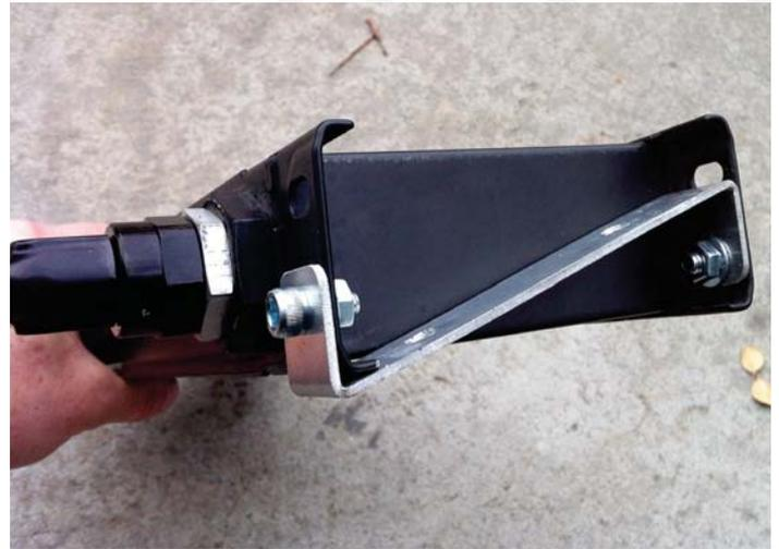
6. Assemble the threaded bush and 'O' ring onto the oil cooler along with the 90o swivel fitting remembering to smear some oil onto the 'O' rings.
