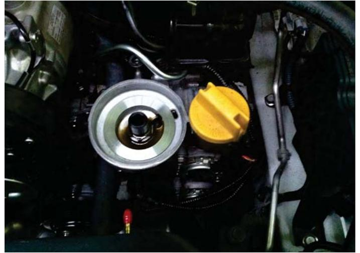
2. Assemble the large 'O' ring to mounting face. Assemble the 'O' ring supplied with the dash fittings to the dash fittings, now assemble the dash fittings to the adaptor using some engine oil to lubricate the 'O' rings.
