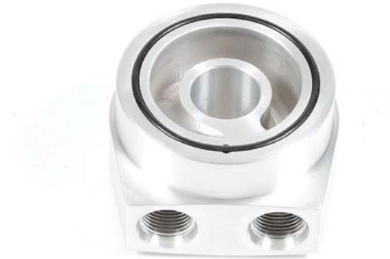
3. Install the sandwich plate on top of the riser plate having smeared some oil on the 'O' ring. Fit and screw the retaining socket to align and hold the two in place. Tighten to 30 Nm torque.
