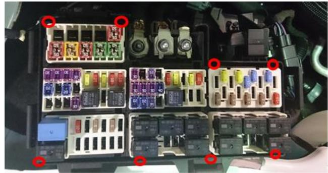
Now that the fuse assembly has been removed, remove the relays in the front right outer section. Now remove the white locking plate as shown in image.
