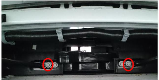
Fit the two U nuts to the front lower rails (inner holes) as per image.
