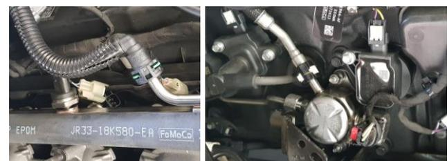
Remove the rubber booster hose the fuel lines and the four heater support brackets using a 10mm socket and place aside. Remove the steel/rubber brake booster line disconnecting it from the booster and place aside, remove the fuel rail foam noise suppressors and place aside.
