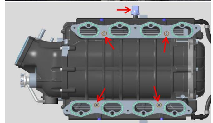
Installing the injectors, for MY18 vehicles transfer these from the NA manifold to the supercharger manifold, injectors supplied for MY15-17 vehicles, ensure the safety clips are also transferred for both variants. Use a suitable lubricant on the O rings of the injectors.
