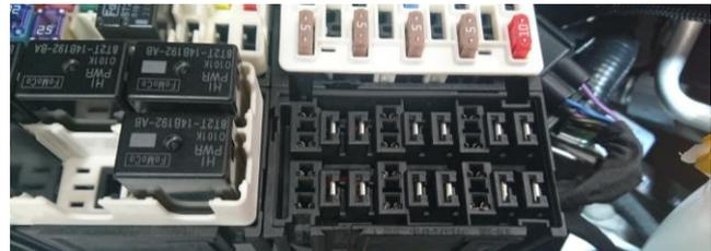
Flip the fuse assembly towards the engine so that access to the underside is achieved. Using the supplied pump loom insert the red wire in the cloth cover as shown (1). Insert the black wire above the red wire (2), insert the red remote fuse wire (3) and finally the red with the eyelet wire (4). Once these have been connected refit the white locking plate.
