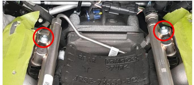
To install the manifold the upper lid needs to be removed from the supercharger to enable the inner 4 screws to be installed. Remove the M6 screws and the 1 M8 securing the by-pass and remove lid assembly. Ensure that the TMAP sensor loom is attached to the manifold and the fuel line connection points are tight.
