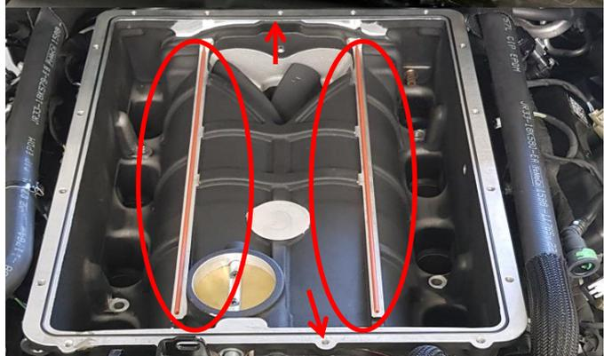
Now install the other 4 screws at the rear of the manifold closest to the firewall using a ¼ drive 5mm hex ratchet set. Once all of these are finger tight, install the remainder of the upper manifold screws. Remember to refit the left and right hose supports and the fuel purge bracket and then torque all upper manifold bolts to **12-14Nm**.
