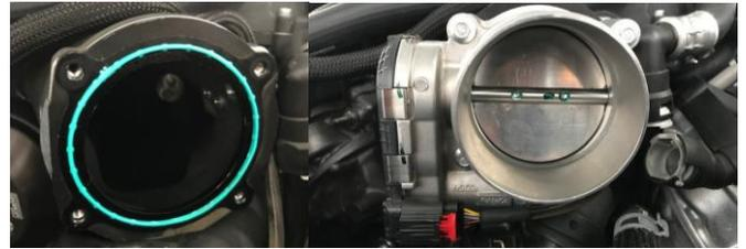
Assemble the Harrop air intake tube to the air intake shield using the screws supplied. Remove the MAF card from the standard air box and install into the Harrop intake tube with the supplied screws. Fit the pod filter to the intake tube. Install the clean air intake tube using the supplied clamps.
