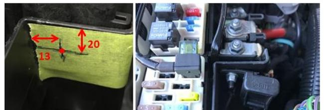
Tuck the loom in under the fuse assembly and fit it back into the box ensuring that the black wire can reach the earth point. The red wire with the eyelet will fit the power as shown in image.
