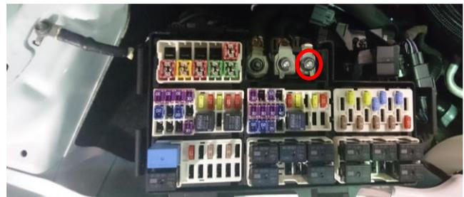
The earth wire is now secured under the screw located behind the ECU.
