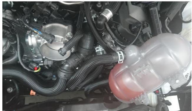
The manifold should now be ready for removal which needs to be done in conjunction with the disconnection of the 4 connectors at the rear of the manifold and the unclipping of two harness ties that are secured to the rear of the manifold.
