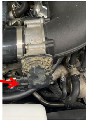
Connect the free end of the 5/16" x 320 long coolant hose to the rear facing barb on the throttle.
