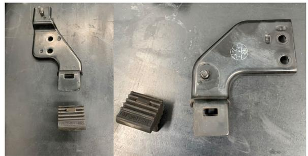
Insert these rubbers into the Harrop Intercooler Radiator #15240 lower brackets.
