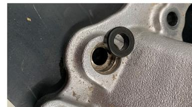
Remove 6x bolts and 4x nuts that secure the Toyota lower manifold to the engine. These will be re-used.
