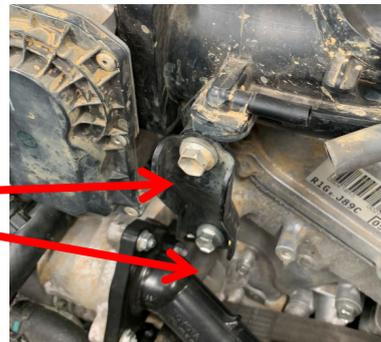
Vacuum out the areas around the inlet manifold bolts to ensure no loose material can fall into the engine.
