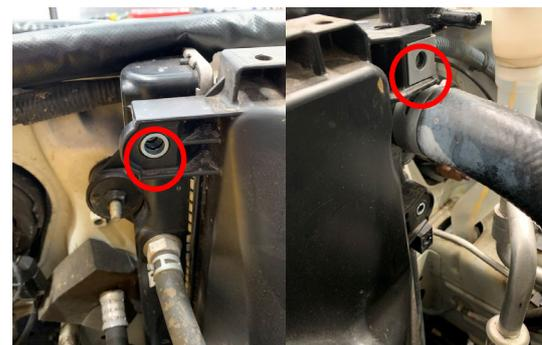
Remove 4x flange nuts that secure the Engine Fan.
