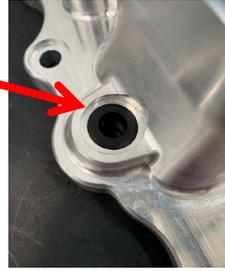
Remove the protective tape and clean the head faces and original intake gaskets, and install the Harrop lower manifold to the engine using the original fasteners. Torque to 22-24Nm.
