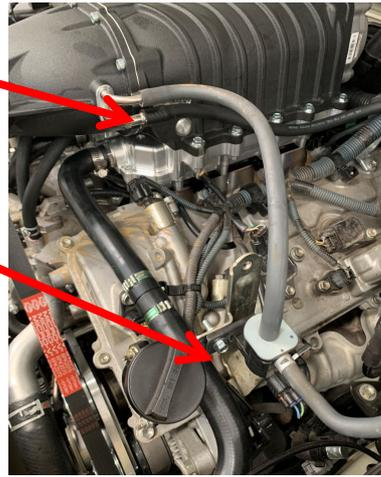
Attach one end of the supplied 3/8" x 500mm long Vacuum hose to the lower elbow on the supercharger LHS and connect the other end to the PCV valve at the back of the LH valve cover.
