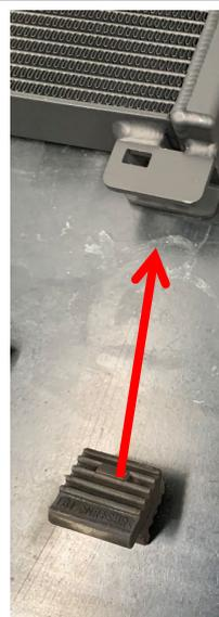
Install the Intercooler Radiator in front of the A/C condenser. Ensure the rubbers on the lower brackets fit over the lip on the lower crossmember.
