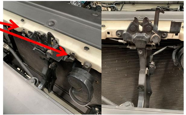
Temporarily remove the hood latch and un-clip the Ambient air temp sensor from the centre strut.
