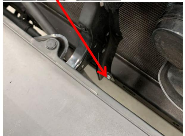
Remove 2x M6 screws and 1x M6 nut from the mount bracket of the lower RHS of the A/C condenser.
