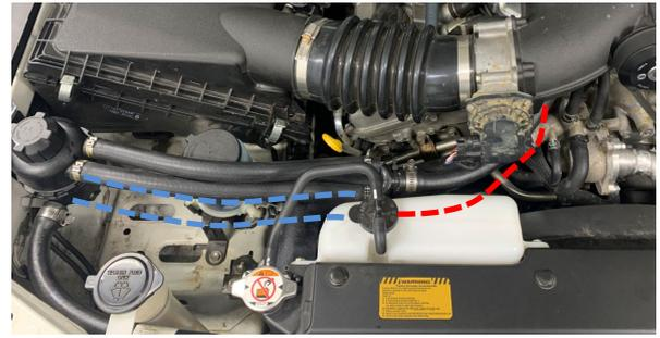
Connect the remaining branch of the Y-piece to the front of the supercharger manifold using the supplied 3/4" x 280mm long intercooler hose shown in red. Secure with 2x hose clamps.
