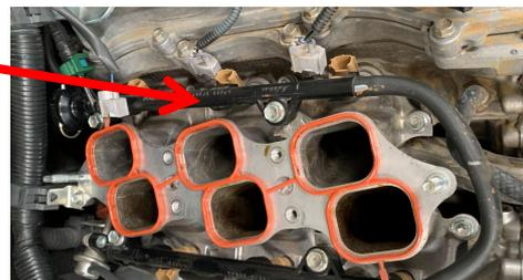
At the rear of the fuel-rails, dis-connect the fuel delivery pipe and the fuel return pipe. Use a rag to wrap the connection before it is separated to prevent residual fuel from spraying out.
