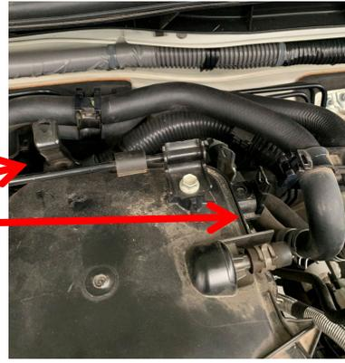
Remove the manifold support bracket from the LHS rear.
