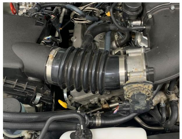
Connect the vacuum hose end to the top elbow on the Supercharger LHS
