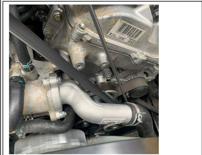
Connect the supplied 5/16" x 380 long coolant hose to the LH hose fitting on the top of the OE water manifold.
