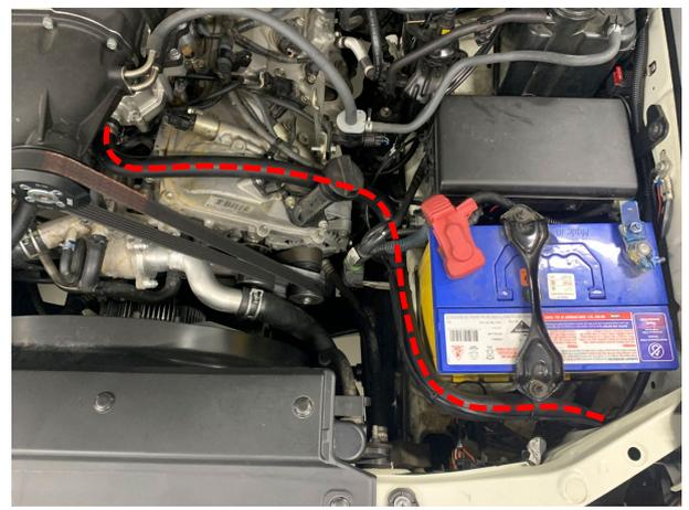
Temporarily remove the plastic trim from the top of the RHS engine bay by removing 5x trim clips and the pulling upwards firmly.
