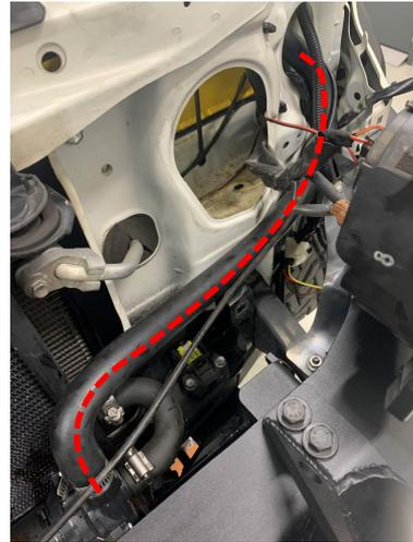
Plug-in the intercooler pump loom #A13128 to the pump and cable tie to secure it along the hose. Run the loom up behind the battery for connection later.
