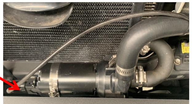
Route the pump outlet hose around the battery, behind the oil filler and across to the LHS intercooler fitting on the front of the supercharger manifold.
