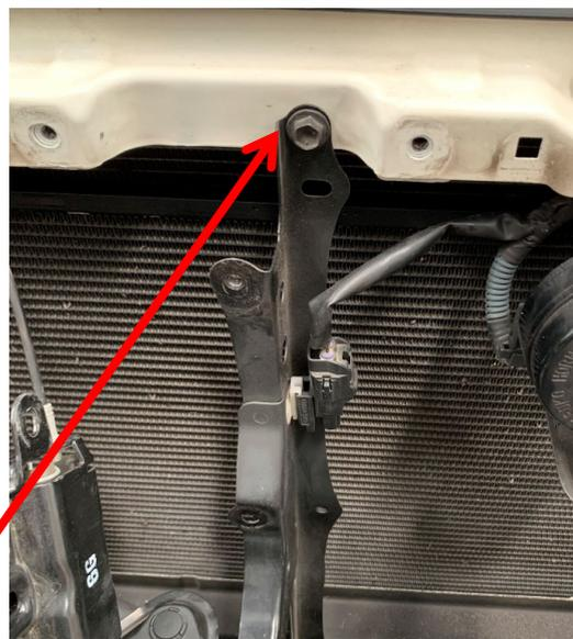
Unbolt the centre strut from the bumper bar and lower crossmember to remove the strut. This will be replaced by the supplied centre strut bracket.
