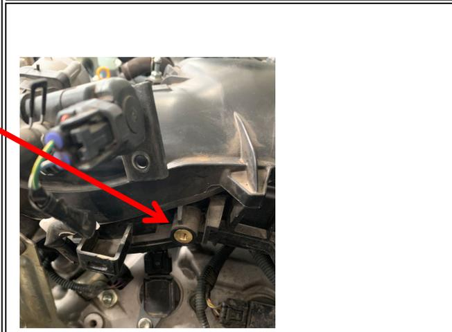
Un-clip the heater hoses from the rear of the inlet manifold in 2 places.
