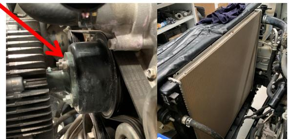
Remove the Crank Pulley Bolt (CCW) using an Impact Gun.
