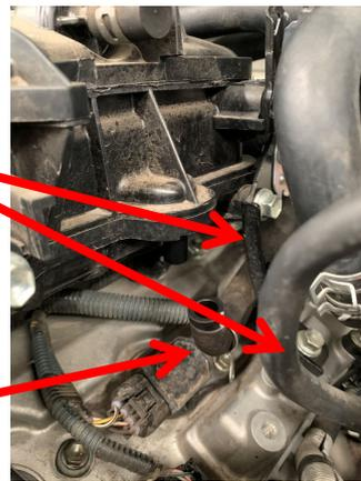
Dis-connect the PCV vacuum hose from under the LHS of the inlet manifold, and remove this hose completely by also disconnecting from the PVC valve at the rear LHS valve cover.
