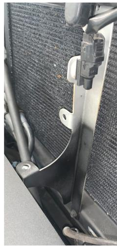
Install the intercooler pump bracket #15308 to the lower cross-member near the LHS of the Intercooler radiator. Screw the bracket to the crossmember using the supplied M6 screws and existing tapped holes. Using the supplied hose clamps, secure the intercooler pump to the bracket with the pump outlet oriented vertically.
