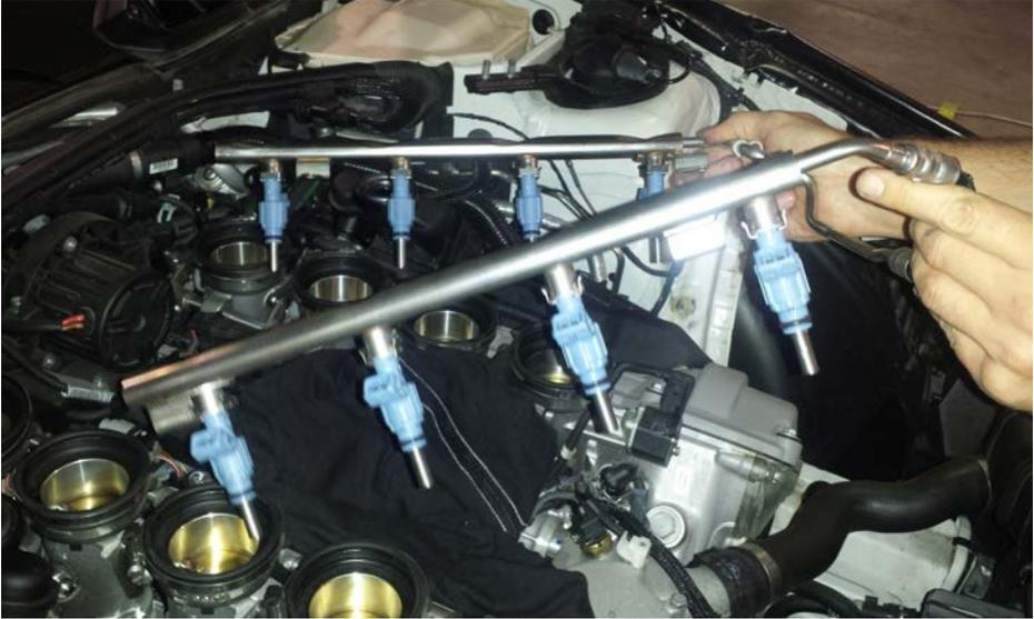
7.c Fit the fuel rails ensuring the injectors are correctly seated in the throttle bodies.
