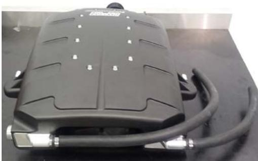
9.b. Install the 860 long molded 16mm hose to the front left hand intercooler fitting using the supplied cobra clamp (21mm green band) this line runs under the front intake of the supercharger assembly.
