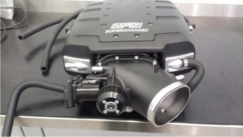
9.c. Install the supercharger assembly. Ensure the throttle body rubbers and the undersides of the supercharger are clean. (Be sure to lift the supercharger assembly into position. Do not slide the assembly over the rubber boots as this may damage or fold them) Before lowering the assembly fully connect the breather line at the front of the engine (Step 4n) to the fitting on the underside of the supercharger inlet.
