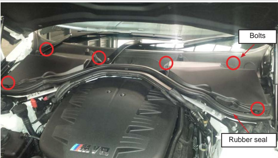
5.c. Remove the left side from the car. Disconnect the alarm loom from the right side and remove the cover from the vehicle.
