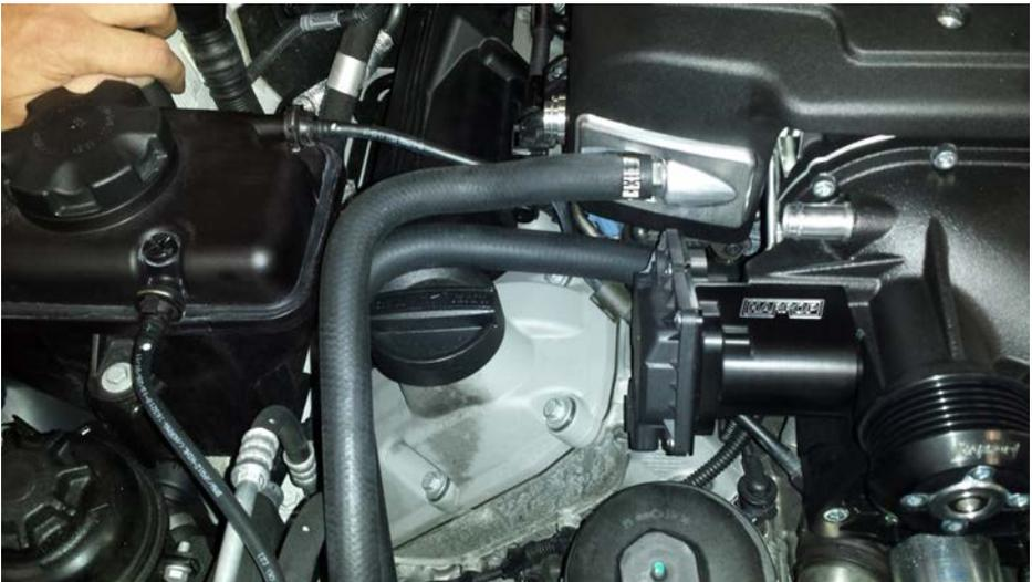
9.j. Remove the IAT sensor from the front R/H side of the standard manifold and install it into the front R/H side of the supercharger manifold. Using the supplied loom extension connect the IAT sensor to the engine harness.
