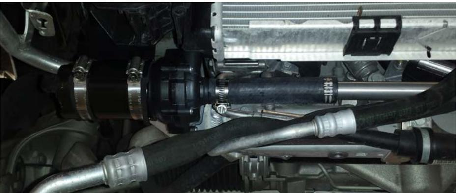
12.s. Install the black “Y” fitting into the front intercooler hoses on the supercharger manifold (21mm green band cobra clamps). Install the 420 long 19mm hose to the other end of the “Y” piece fitting and secure with a cobra clamp (white band).
