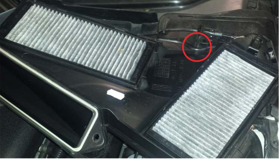
5.d. Remove the 3 bolts securing the loom harness. (Found on right hand drive built cars)
