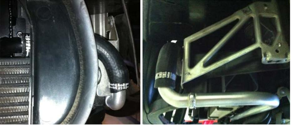
12.p. Install the 125 long 19mm hose to the straight end of the long intercooler pipe using a cobra clamp (white band).
