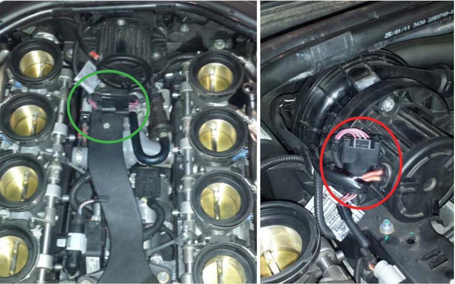
7.g. Remove the standard purge line from manifold vacuum to the purge solenoid, remove the solenoid mount.
