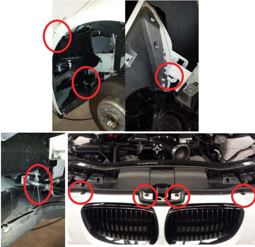
12.d. Remove the air duct from above the radiator. Remove the 2 scrivets and lift the duct off.
