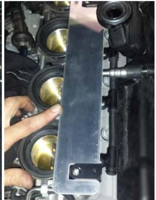
7.e. Reconnect the injector loom ensuring the spring clips snap in place.
