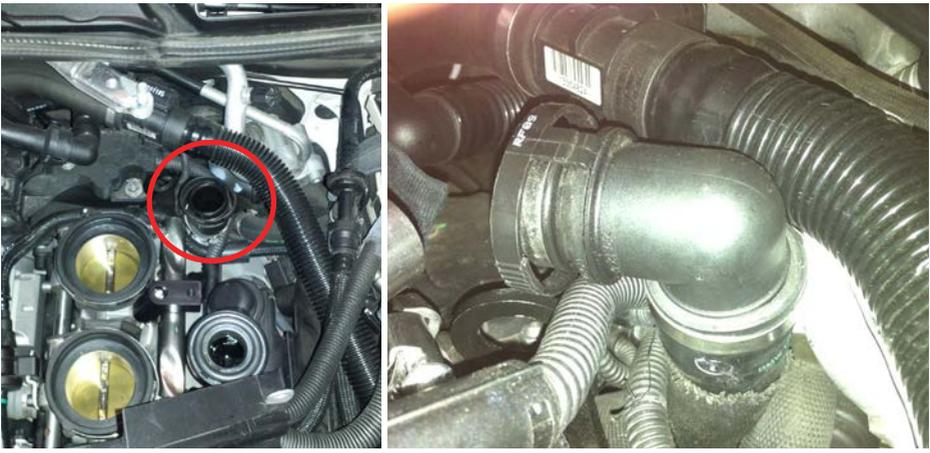
7.l. Remove the engine lifting bracket from the front R/H side of the engine, shown in green, this will not be refitted (2 x 8mm torx bolts). The breather line located at the front L/H side of the engine requires shortening (shown in red below). Trim 75mm off the end of this hose.
