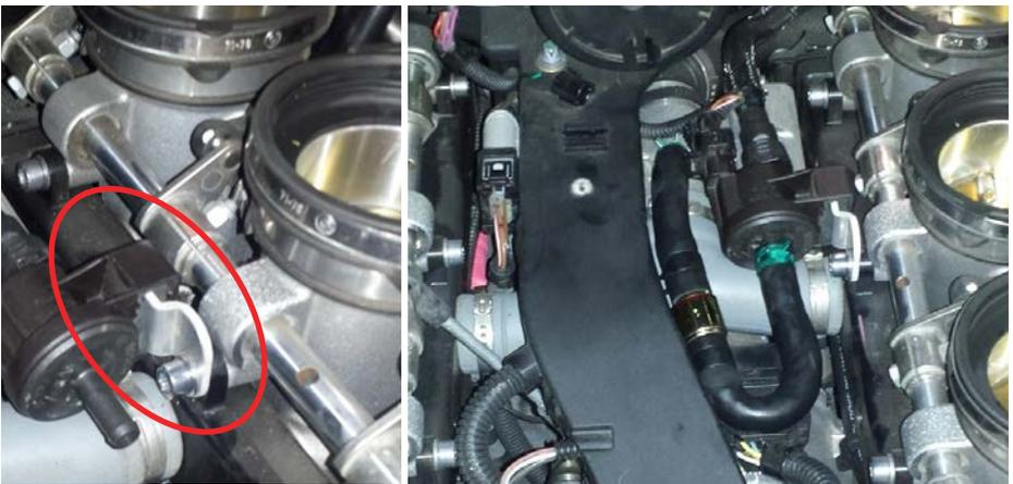
7.k. Remove the 45 degree quick connect fitting from the idle air circuit line (rear L/H side) and replace with the supplied 90 degree quick connect fitting.
