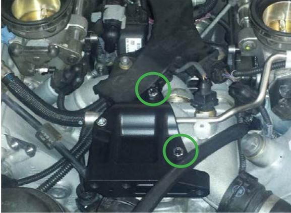
8.h. Remove the FEAD assembly (6 by M8 cap screws, be careful not to move the above supercharger FEAD mount)
