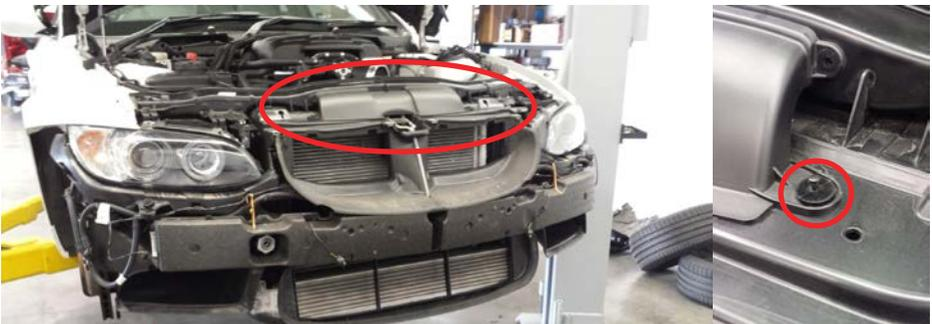
12.e. Remove the 3 torx bolts securing the bonnet catch and rubber grill surround. Unclip the rubber grill surround and remove together.
