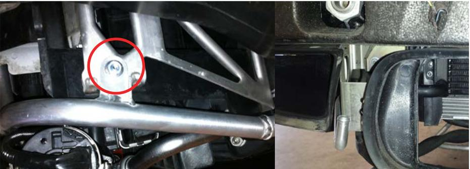
12.l. Loosen the 2 nuts above and the 2 nuts below on the R/H side of the radiator that mount the radiator support panel to the sub frame.
