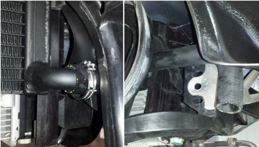
12.o. Install the 900mm long intercooler pipe to the L/H side of the intercooler radiator hose using the supplied cobra clamp (white band).
