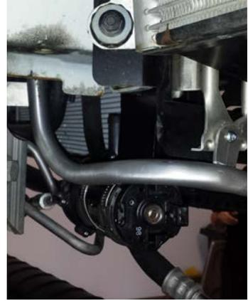
12.n. Fit the 2 short 90 degree 19mm bend hoses to the front of the intercooler, long ends on intercooler short ends pointing down. Secure with cobra clamps (white band).
