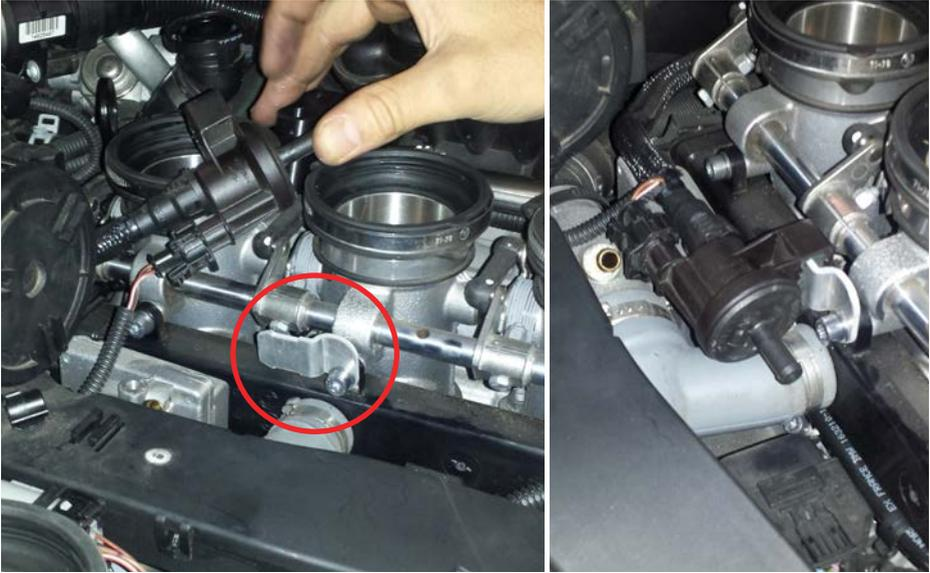
7.i. Use the supplied zip tie to secure the purge solenoid to the mounting bracket.
