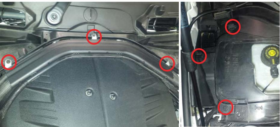
5.f. Remove the nut supporting the wiring harness on the right hand side strut brace.
