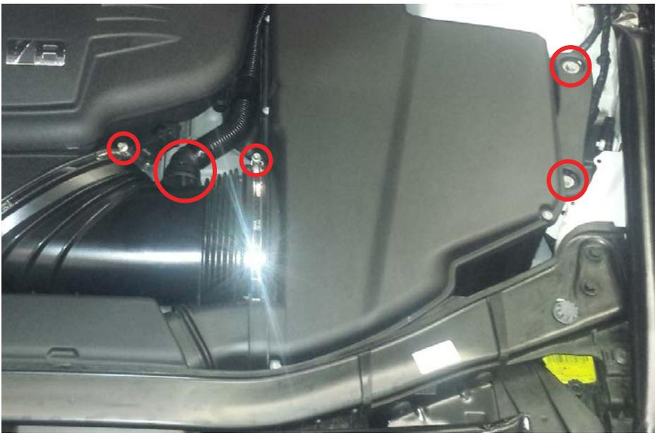
4.d. Lift the air box up off two grommets to remove it from the engine bay.
