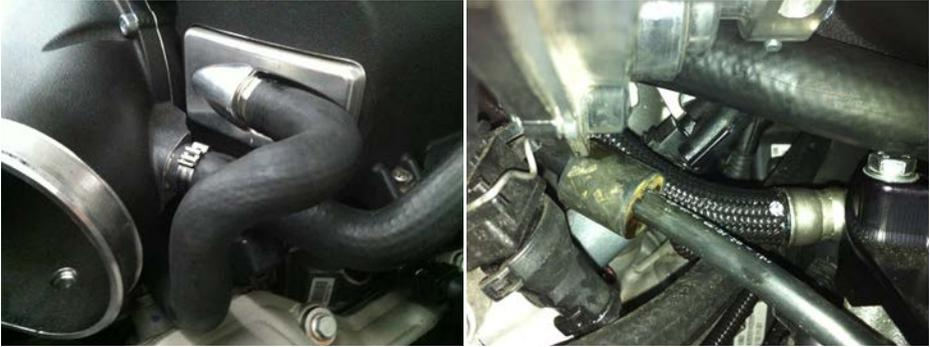
9.e. Visually check that the rubber throttle body boots are in the correct position and are not folded.
