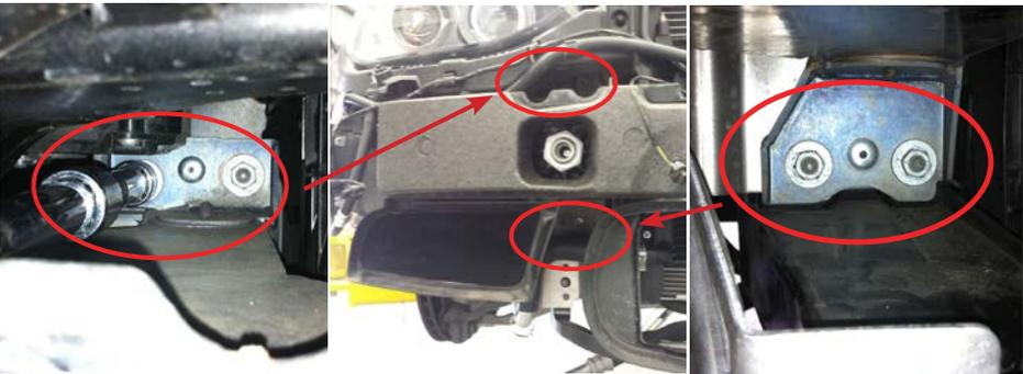
12.m. Assemble the intercooler pump onto the pump bracket with the outlet pointing upwards as shown below. Slide it up between the end of the chassis rail and the radiator support panel until the slots bottom out on the radiator support panel studs. Once the pump assembly is in position re-tighten the 4 radiator support panel nuts.
