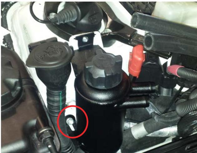
12.x. Install 390 long 19mm intercooler hose between the lower fitting on the reservoir bottle and intercooler pipe running to the right hand side of the intercooler radiator. Fit the supplied worm drive clamps both ends.
