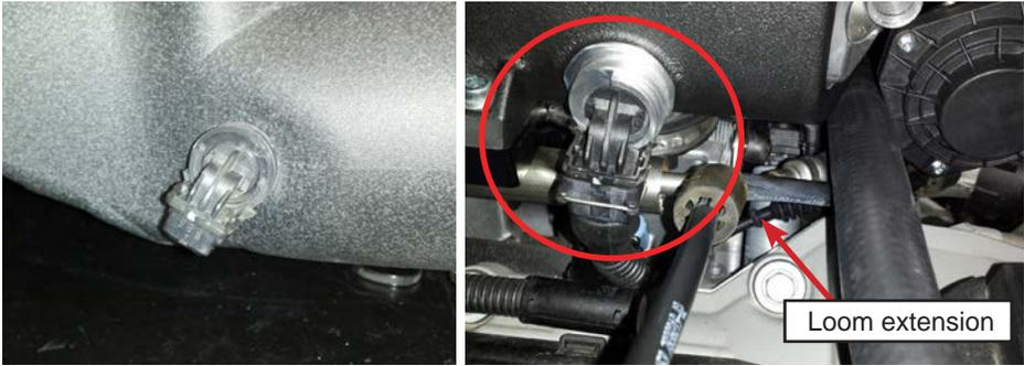
9.k. Connect the newly fitted 90 degree quick connect on the idle air circuit hose to the rear L/H side of the supercharger manifold.
