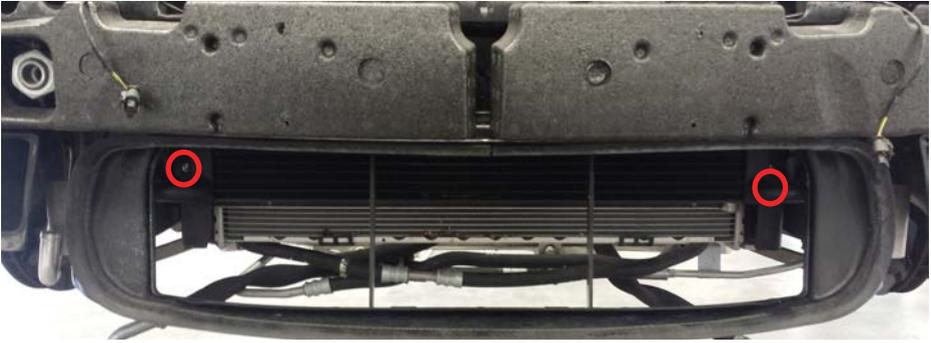
12.k. Install intercooler pipe to the R/H side of the intercooler radiator using the supplied M6 button head / flange nut.
