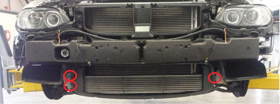
12.h. Install the intercooler radiator by sliding it up from under the vehicle until the pin is fully inserted in the grommet installed previously. The bleeder nipple should be on the R/H side of the car.
