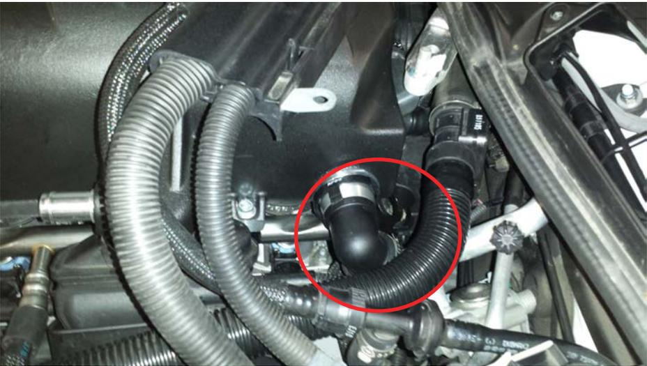
9.l. Install the supplied valve cover molded breather hoses to the valve covers / supercharger inlet as shown below. Secure with 4 cobra clamps (black band).
