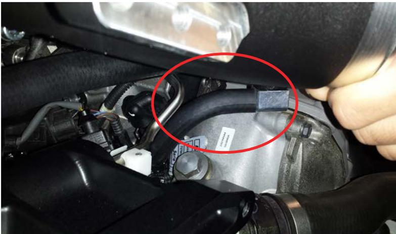
9.d. Lower the supercharger assembly into position checking the routing of the L/H intercooler line is as shown below, ensure its clear of the throttle linkage on the R/H front throttle body.
