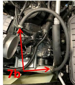
**7.c)** Connect the remainder of the  $\varnothing$  5/16" coolant hose between the lower elbow on the throttle body and the barb on the thermostat housing. Secure with the OE spring-band clamps.
