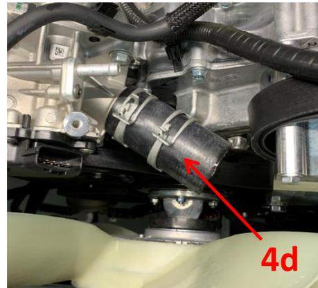
**4.e)** Insert the radiator hose assembly into position and then insert into the reducer hose.
