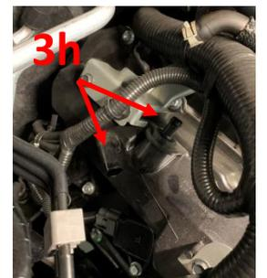
**3.i)** Remove the flexible intake tube from between the Throttle body and Airbox. Unclip the airbox lid to make this easier.
