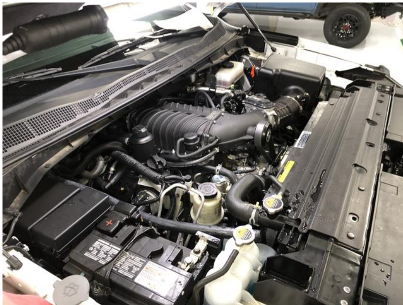
Harrop TVS2300 Supercharger kit installed on a 2019 Nissan Titan
