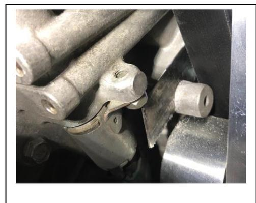
**4.c)** Swap the lower radiator hose and coolant temp sender to the Harrop hard-line. Re-use the OE spring-band clamps.
