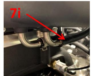
7.j) Using the remainder of the  $\text{\O}3/8''$  PCV hose, connect the RH valve cover to the fitting on the RHS of the supercharger inlet.
