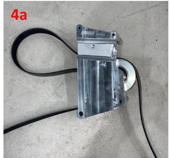
**4.b)** Remove 3x M6 screws from the LH timing cover that will be replaced with the Idler bracket screws. Install the idler bracket and belt together to the front of the engine, ensuring that the belt is not wrapped around the lower post of the bracket.
