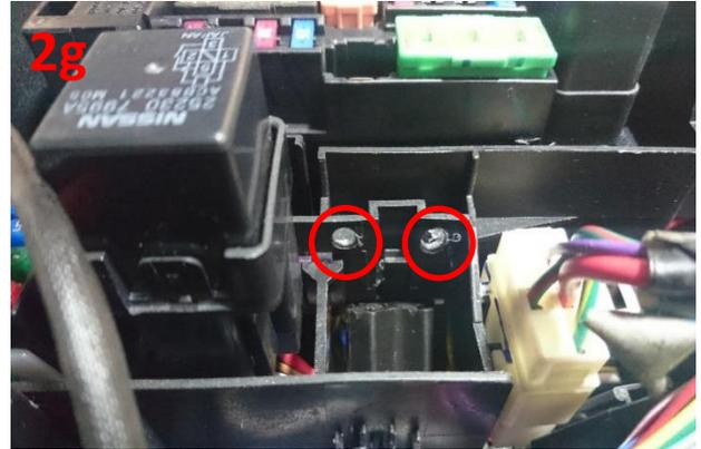
**2.h)** Once the holes have been drilled thread the supplied cable tie through the holes and secure the relay connector in position.
