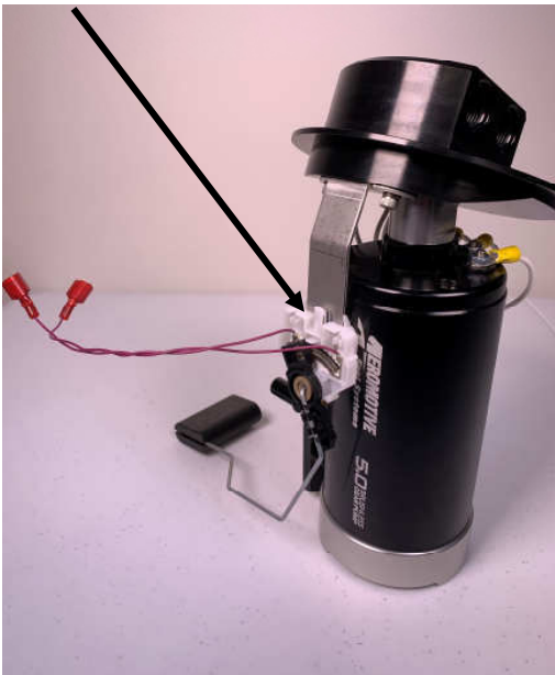
Fuel Level Sensor properly installed on bracket.
