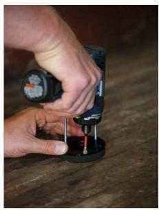
8. Once four of the screws are started, remove the two studs and insert the two remaining screws in the holes. Now fully tighten the filler cap screws, they just need to be tight enough to compress the gasket and sit flush against the mounting surface. Do not overtighten the screws to avoid damaging the housing.
