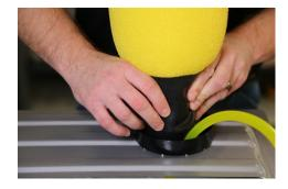
9. On the bottom of the Phantom pump hanger assembly, replace the 1/8 NPT plug in the outer outlet port (the pump is connected to the center port) with the new fuel jet siphon assembly. Note the approximate orientation of the siphon inlet barb in the following figure (this will aid in installation).
