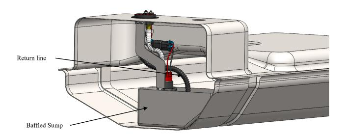
9. Install either ORB-06 x AN flare 90-deg fittings with the AN male sized to match your fuel lines (for AN-06 line use Fragola PN 499206BL; for AN-08 line use Fragola PN 499207BL, or other like fittings).
