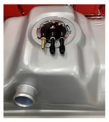
8. Connect the supply and return fuel lines to the new Aeromotive fuel pump assembly. The supply and return fittings are AN-06 male flare and will require AN-06 female hose ends. The vent port is a ¼" hose barb in which the OEM vent hose can reattach to. Note: AN-08 lines will be required for carbureted applications; AN-06 or AN-08 lines may be used for EFI applications.
