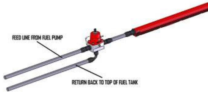
Fuel Rail with single inlet (Figure 1-1)
