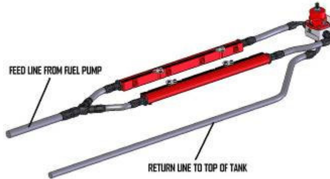
Fuel Rails with inlet/outlets (Figure 1-2)
