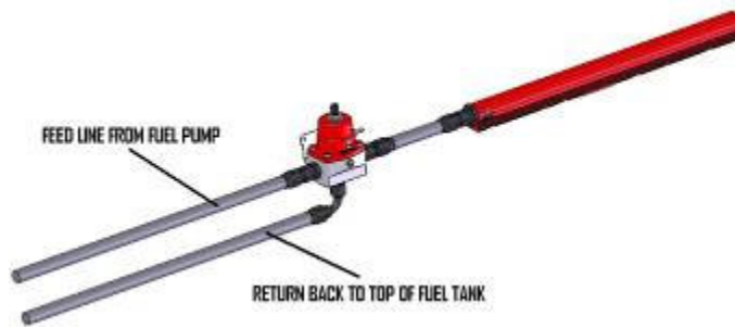
Fuel Rail with single inlet (Figure 1-1)
