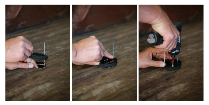
20. Once four of the screws are started, remove the two studs and insert the two remaining screws in the holes. Now fully tighten the filler cap screws, they just need to be tight enough to compress the gasket and sit flush on the bed floor. Do not overtighten the screws to avoid damaging the housing. Next, install the fuel filler cap using the provided key. See pictures below.
