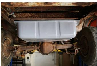
26. Once the tank is secured and the filler neck is aligned with the filler hose, reach in behind the bed crossmember and tighten the lower hose clamp with a 5/16 nut driver. See picture below.
