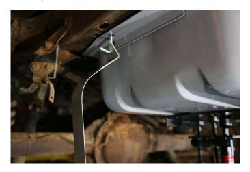
25. On the opposite side of the tank from the "J" bolts, use the two 3/8 bolts to tighten the straps up to the tank. See pictures below.
