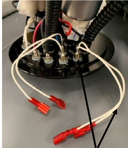
Two wires soldered to common terminal used for fuel level sender(s) ground "LVL -".
