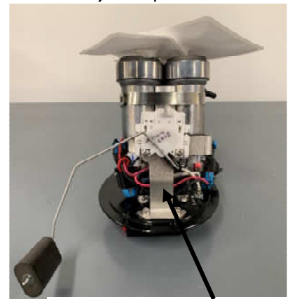
Installed "New-Style" fuel level sender bracket on outlet cap with socket head cap screws and lock washers.
