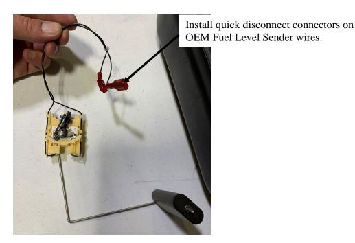
16. Install OEM Fuel Level Sender on Fuel Level Sender Bracket. First remove the Fuel Level Sender Retainer from the Bracket by loosening the two 6-32 screws/nuts. Once the retainer is removed, slide the OEM Fuel Level Sender onto the bracket by lining up the grooves on the side of the OEM Fuel Level Sender with the "legs" of the Fuel Level Sender Bracket.
