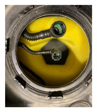
12. Pull the Siphon Adapter Hose up and over the Foam and Fuel Baffle assembly with the end sticking out of the fuel pump hole.
