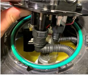
22. Connect the white LVL wires with the wires from the OEM Fuel Level Sender using the quick disconnect connectors. **Note:** It doesn't matter which wires are connected to each other as the circuit is resistance based.
