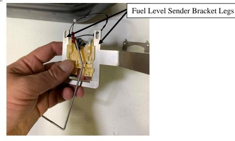
17. Slide the OEM Fuel Level Sender down until it bottoms out in the Bracket groove. Then install the Fuel Level Sender Retainer using the provided 6-32 screws, washers, lock washers, and nuts. Note: Ensure the OEM Fuel Level Sender is installed as shown in the picture otherwise it will not be oriented correctly in the tank and will result in an incorrect fuel level readings.
