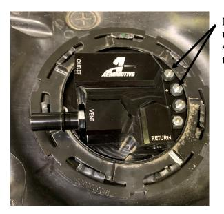
Note: Aux. Terminals are not used in this application and should have no wires connected to them.
