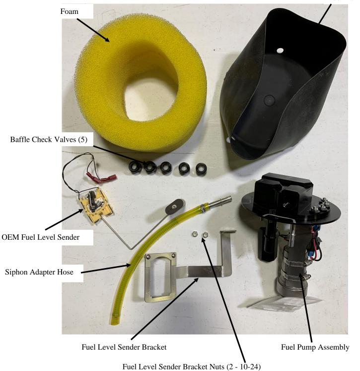
8. Insert Check Valves into Fuel Baffle. Insert the tapered end of the Check Valve from the inside of the Fuel Baffle through each of the 5 holes. Push the Check Valve through the hole until it is retained by the small groove.
