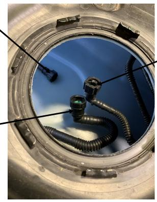
Gas Recirc Line Connector (5/16" Quick Connect)
