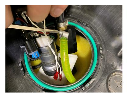
21. Connect the Gas Recirc Line to the 5/16" quick connect fitting on the underside of the Fuel Pump Assembly outlet cap, then connect the Tank Vent Line to the 5/8" quick connect fitting on the underside of the Fuel Pump Assembly outlet cap.
