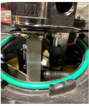
25. Push the Fuel Pump Assembly down into the tank and rotate the outlet cap until the markings with the "J" are lined up as shown in the following image with the arrow on the tank. Secure the outlet cap to the tank with the OEM lock ring.
