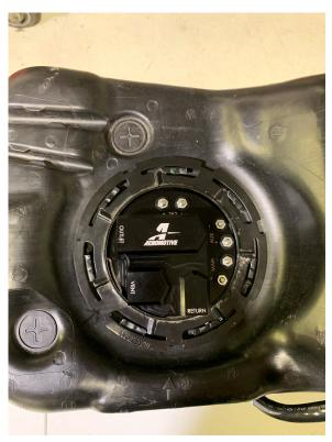
26. Install the provided 5/8" quick connect fitting into the Vent port on the outlet cap. Note: Although the OEM Tank Vent and Fuel Recirc Lines are connected internally in the tank to the bottom of the outlet cap, new or manipulated lines will need made/sourced by the Installer to allow for optimal connections to the outlet cap ports.
