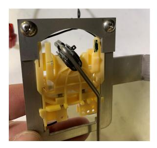
18. Loosely insert the Fuel Level Sender Bracket/Sender assembly into the tank over the top of the Foam assembly, the Level Sender should be pointing towards the front of the tank. Once inserted, let the Fuel Level Sender Bracket attachment flange hang on the edge of the hole as shown in the following images.
