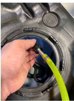
11. Once Siphon Adapter Hose is connected to the OEM siphon pickup tube, insert the Foam/Fuel Baffle/Check Valve assembly into the tank. The Foam and Fuel Baffle assembly should be concentric with the OEM fuel pump assembly hole. Arrange the tank vent line and gas recirc line so they are on top of the Foam and Fuel Baffle assembly.
