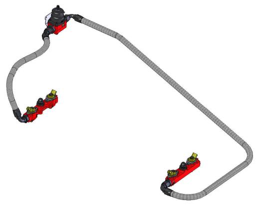
36. Install one ORB-06 o-ring over the male flare and up the shoulder of an AN-06 to 5/16 barb adapter fitting. Install the AN side of this fitting into the supply tee adapter fitting. Locate the assembled tee adapter fitting where it will connect to the OEM fuel supply hose.
