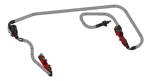
38. Connect one of the AN-08 90-degree hose ends to the top center port on the passenger side fuel rail and a second AN-08 90-degree hose end to the remaining AN-08 male on the supply line tee adapter fitting. Plan a route for the line between the fuel rail and the tee fitting, measure the length of fuel line needed and cut. See section titled Hose and Fitting Assembly for fuel line assembly instructions. Once the hoses are assembled, **ensure there is no debris in the hose** and install it.
