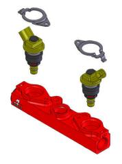
21. Reinstall the injector retaining clips and tighten screws.
