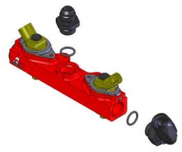
32. Thread the o-ring side of two of the ORB-08/AN-08 port fittings into the top center port, and in the front port, of the driver side fuel rail.
