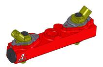
22. Inspect the fuel injector pipe insulators and replace if needed. Install each of the sealing washers on the bottoms of the fuel rail.
