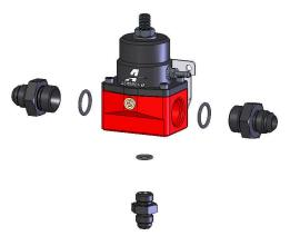
29. Install one ORB-08 o-ring on each of the two ORB-08/AN-08 port fittings.
