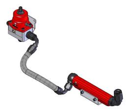
36. Connect one of the AN-06 45-degree hose ends to the Banjo fitting located on the rear of the driver (left) side fuel rail and an AN-06 straight hose end to remaining inlet (side) port on the fuel pressure regulator. Plan a route for the line between these hose-ends, measure the length of fuel line needed, and cut. See section titled Hose and Fitting.
