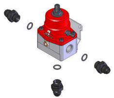
28. Locate the two p/n 15636 ORB-08/AN-06 Banjo Port Fittings and insure that an ORB-08 O-ring is installed on the port Side of each.
