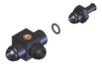
38. Connect the AN-08 straight hose end to the straight-through AN-08 male flare on the supply tee adapter. Plan a route for the line between the supply tee adapter and the AN-08 90-degree male ORB Hose end located in the front of the passenger (right) side fuel rail. Measure the length of fuel line needed and cut. See section titled Hose and Fitting Assembly for fuel line assembly instructions. Once the hoses are assembled, **ensure there is no debris in the hose** and install it.
