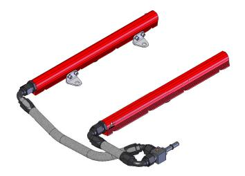
24. Connect one AN-08 90-Degree Male ORB hose end to the rear of each fuel rail. Plan a route between the two hose ends, measure the length of fuel line needed and cut. See section titled Hose and Fitting Assembly for fuel line assembly instructions. Once the hoses are assembled, **ensure there is no debris in the hose** and install them.
